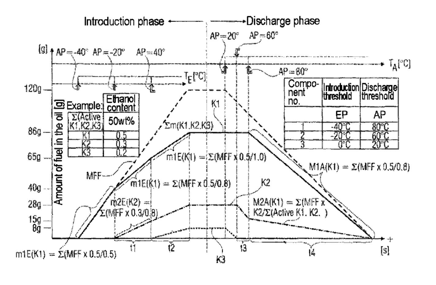
component, which are determined based on a) an introduction parameter in the introduction phase or a discharge parameter in the discharge phase, and b) the first portion of the first fuel component and the second portion of the second fuel component in the fuel.
