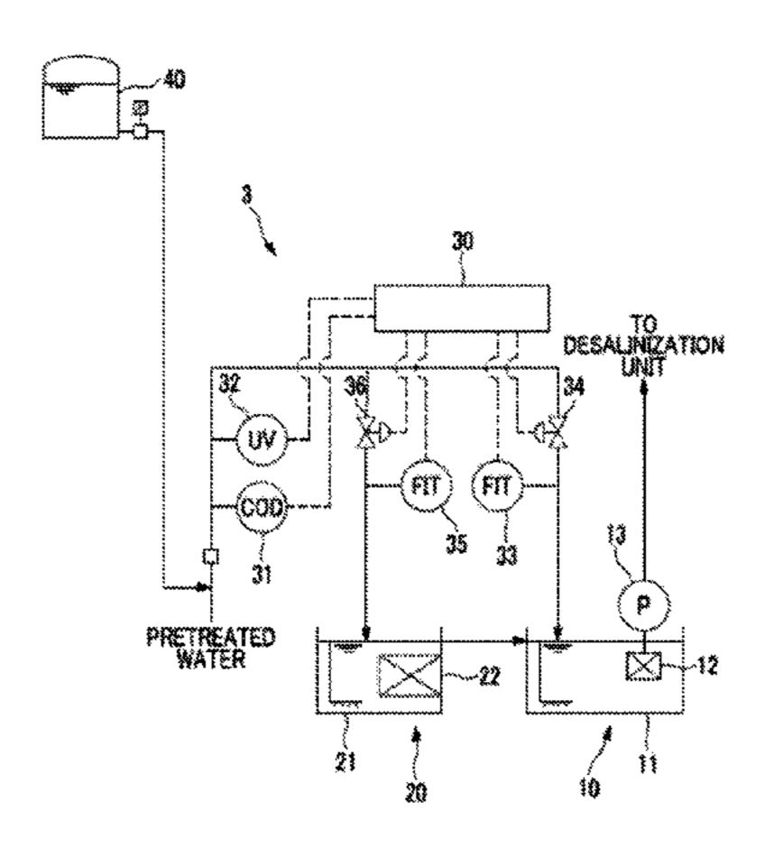
wastewater supplied to the first biological treatment device (10) and a flow rate of the wastewater supplied to the second biological treatment device (20), and adjusts the flow rate of the wastewater supplied to the first biological treatment device (10) and the second biological treatment device (20), based on the distribution ratio.
