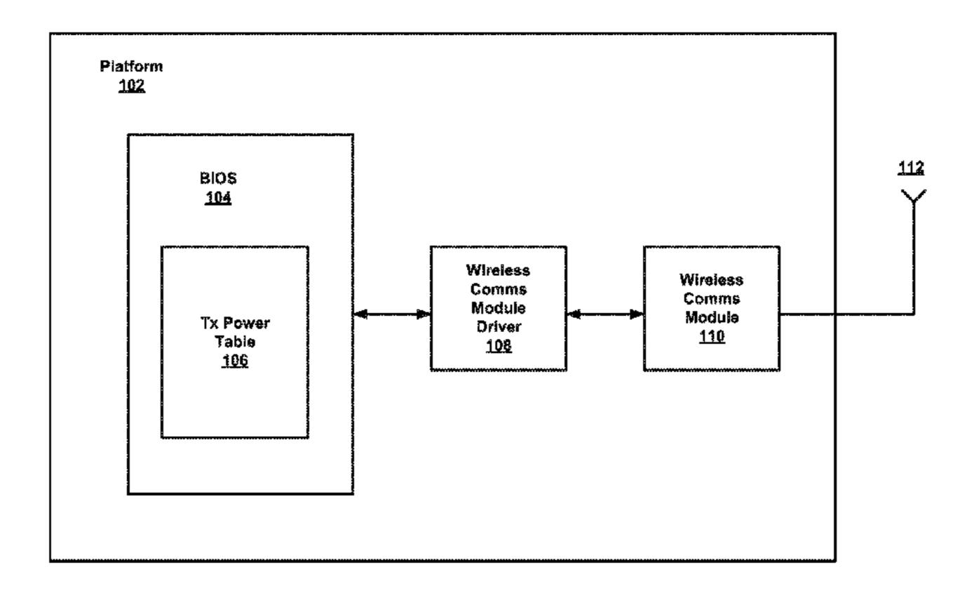
third Tx power level based on a comparison of the first Tx power level and the second Tx power level. The device may further include a radio frequency (RF) transmission module to transmit a wireless signal at the third Tx power level.
