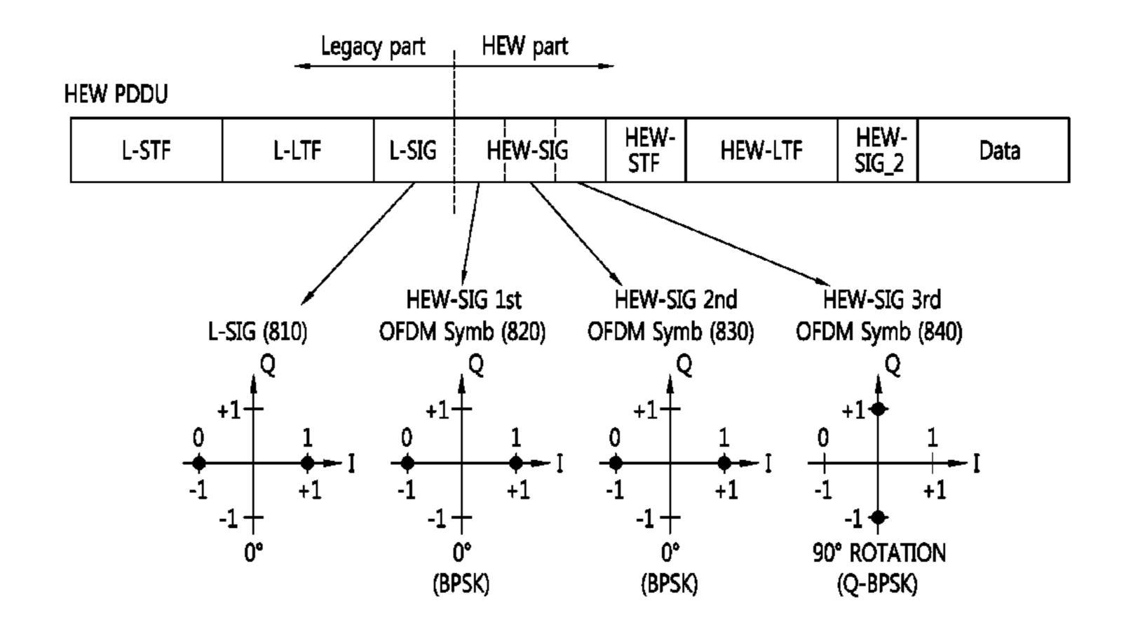
a third OFDM symbol, wherein at least one of a second binary phase shift keying used in the second OFDM symbol and a third binary phase shift keying used in the third OFDM symbol can be rotated in reference to the first binary phase shift keying used in the first OFDM symbol.
