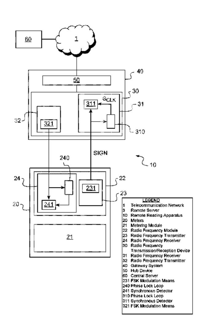
of receiving the signal transmitted according to the modulation, comprising operations of generation of a synchronization signal synchronized with the received signal and synchronous detection of the received signal using the synchronization signal.
