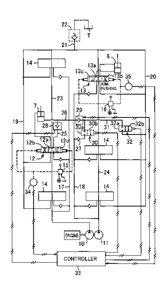
tion action and a second flow path supplying the return oil to the control valve for the specific hydraulic actuator to stop the regeneration action.
