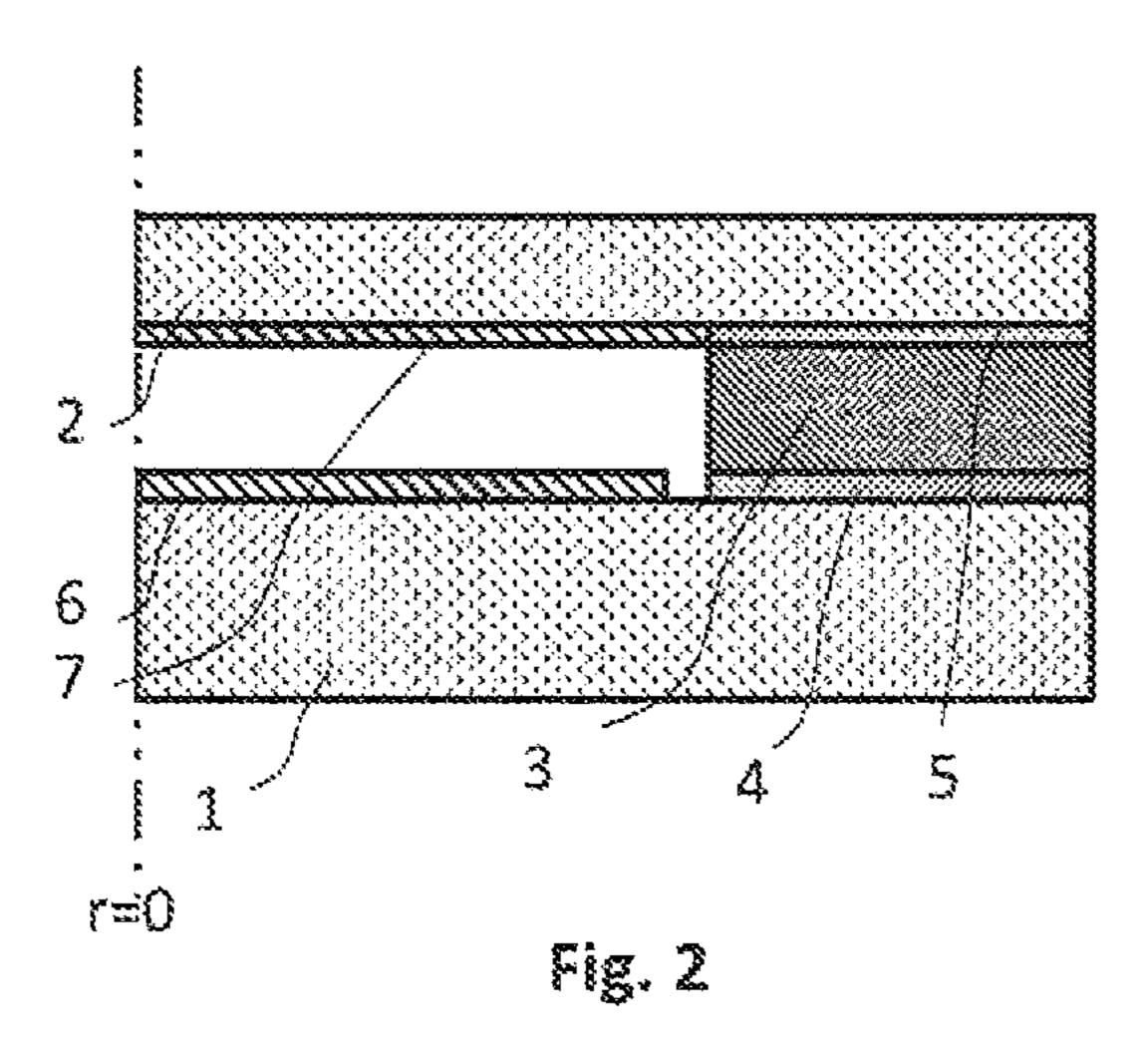
ASSEMBLY HAVING AT LEAST TWO CERAMIC BODIES JOINED WITH ONE ANOTHER, ESPECIALLY A PRESSURE MEASURING CELL, AND METHOD FOR JOINING CERAMIC BODIES BY MEANS OF AN ACTIVE HARD SOLDER, OR BRAZE
