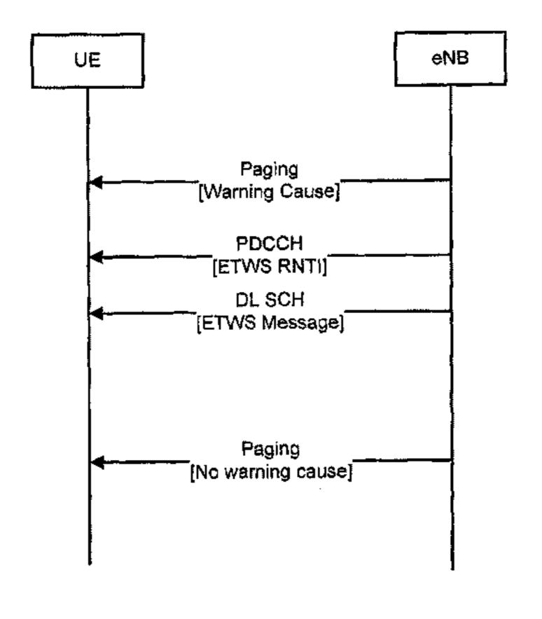
control channel, the system information including scheduling information for the ETWS message, and transmit the ETWS message through a downlink channel according to the scheduling information.
