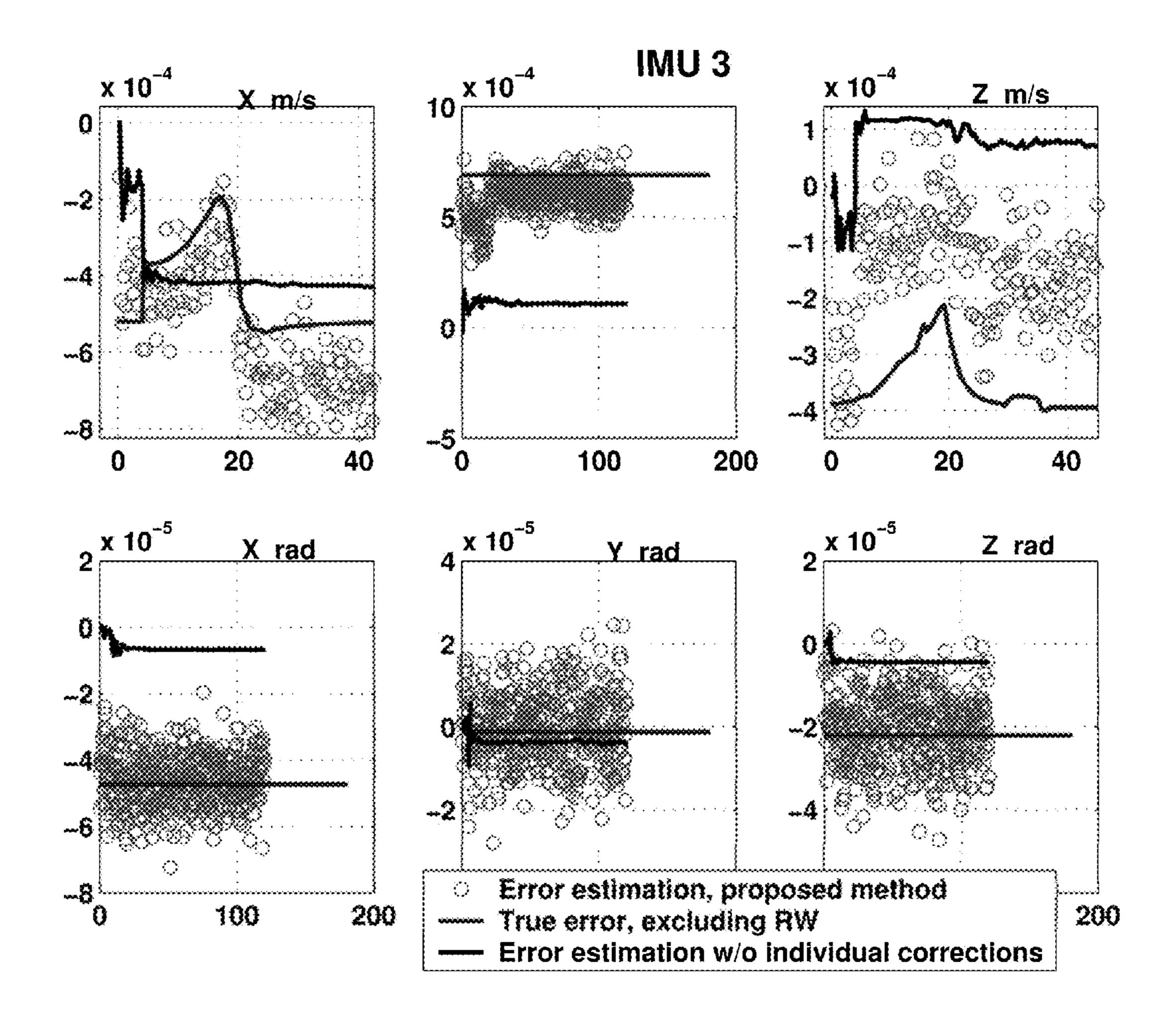
Figure 7: Off-center IMU errors: true, and estimated by both methods
