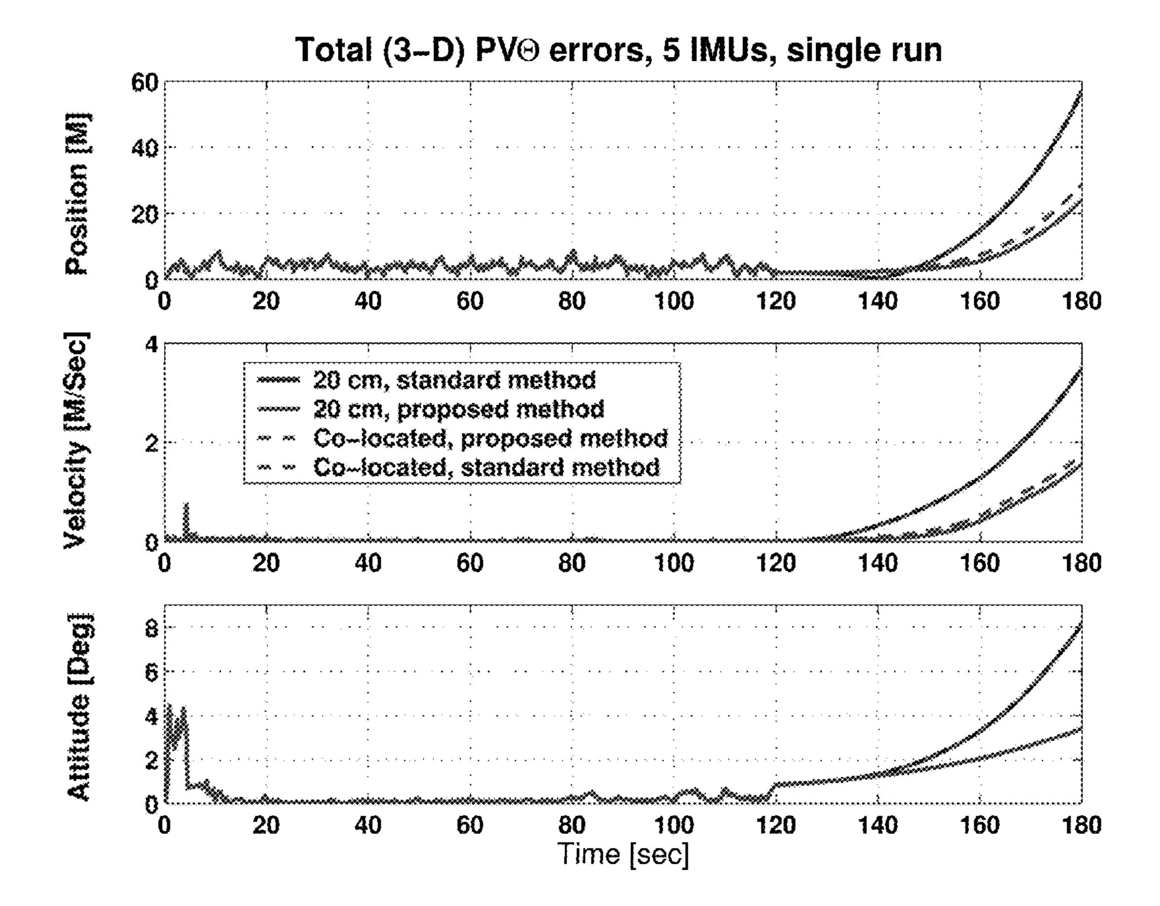
Figure 5:  $PV\Theta$  errors, single run, 2 NAV schemes, 2 HW configurations
