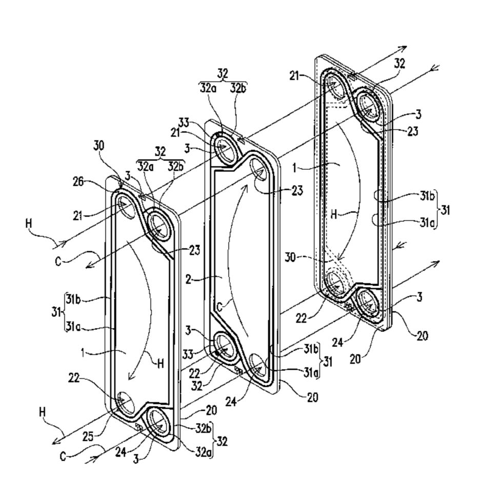
ture fluid H and the low-temperature fluid C, respectively, to flow in and out of the first flow path 1 and the second flow path 2 are formed alternately on opposite sides of each of the heat transfer plates 20. The flow-path forming gasket 31 is made up of an inner gasket member 31a and an outer gasket member 31b arranged in two parallel lines.
