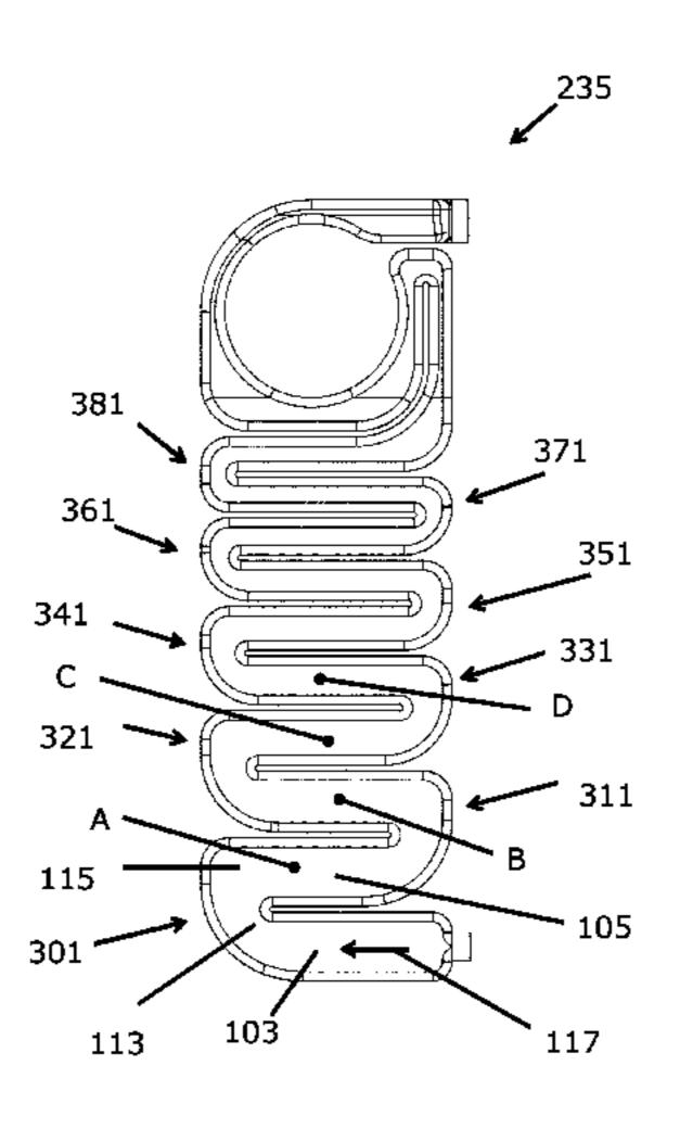
parallel with the width direction of the water flow channel and which is perpendicular to the plane of the wall separating the two consecutive parallel straight segments. In at least two U-turns the upstream section has a volume that is at least 20% lower than the volume of the downstream section.
