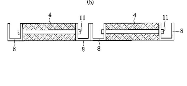
opening or the access way. The door body 2 is formed from a hard polyurethane foam 4 in the form of a sheet.
