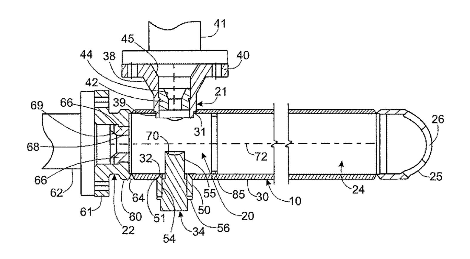
impingement pin for defining an annular ledge for directing a peripheral portion of pressurized gas stream and liquid atomized in the mixing zone radially inwardly for facilitating continued intermixing of the liquid and pressurized gas stream as they proceed through the barrel zone for discharge from the spray nozzle.
