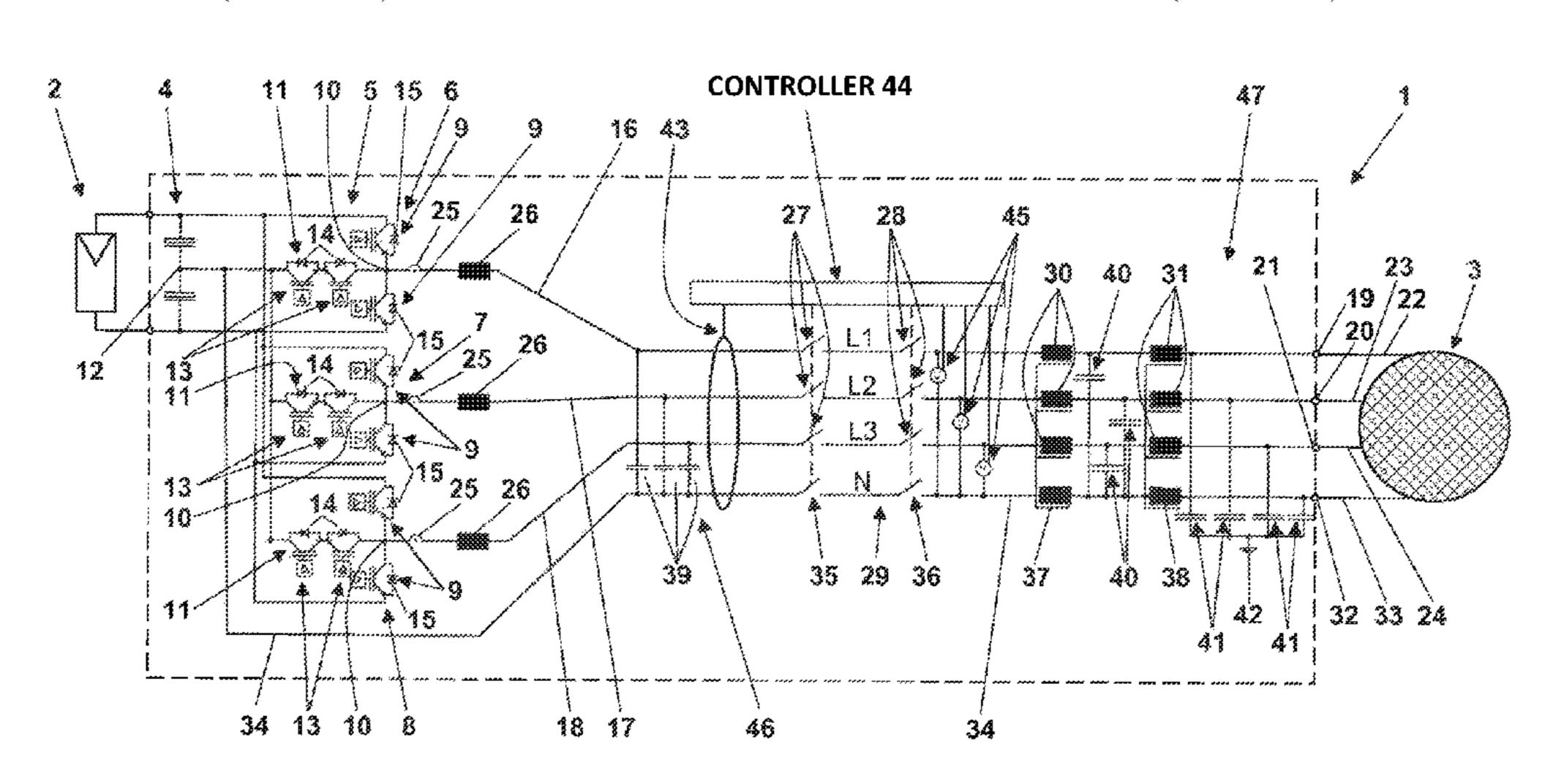
to second operating conditions different from the first operating conditions. The method further includes feeding electric power from the DC intermediate circuit into the AC grid by the inverter bridge with the switch open when the second operating conditions are present, and closing the switch when there is a transition from the second operating conditions to the first operating conditions.
