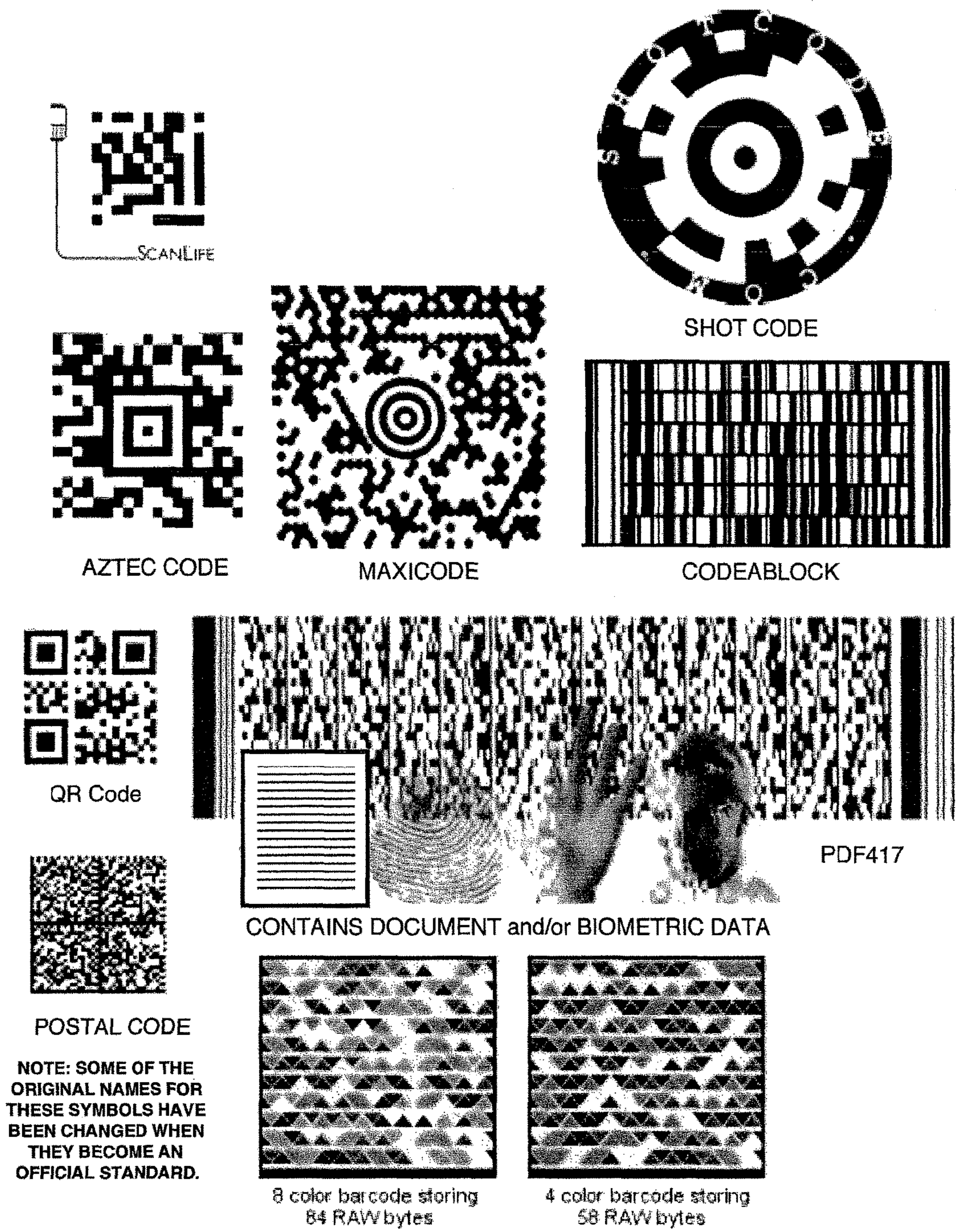
Figure 22A Examples of Different Two-Dimensional Machine-Readable Symbols
