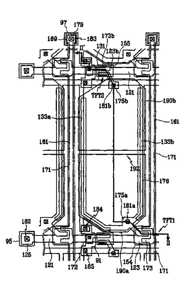
terminals connected to a previous gate line, a storage electrode line or one of the data lines, and one of the second pixel electrodes.
