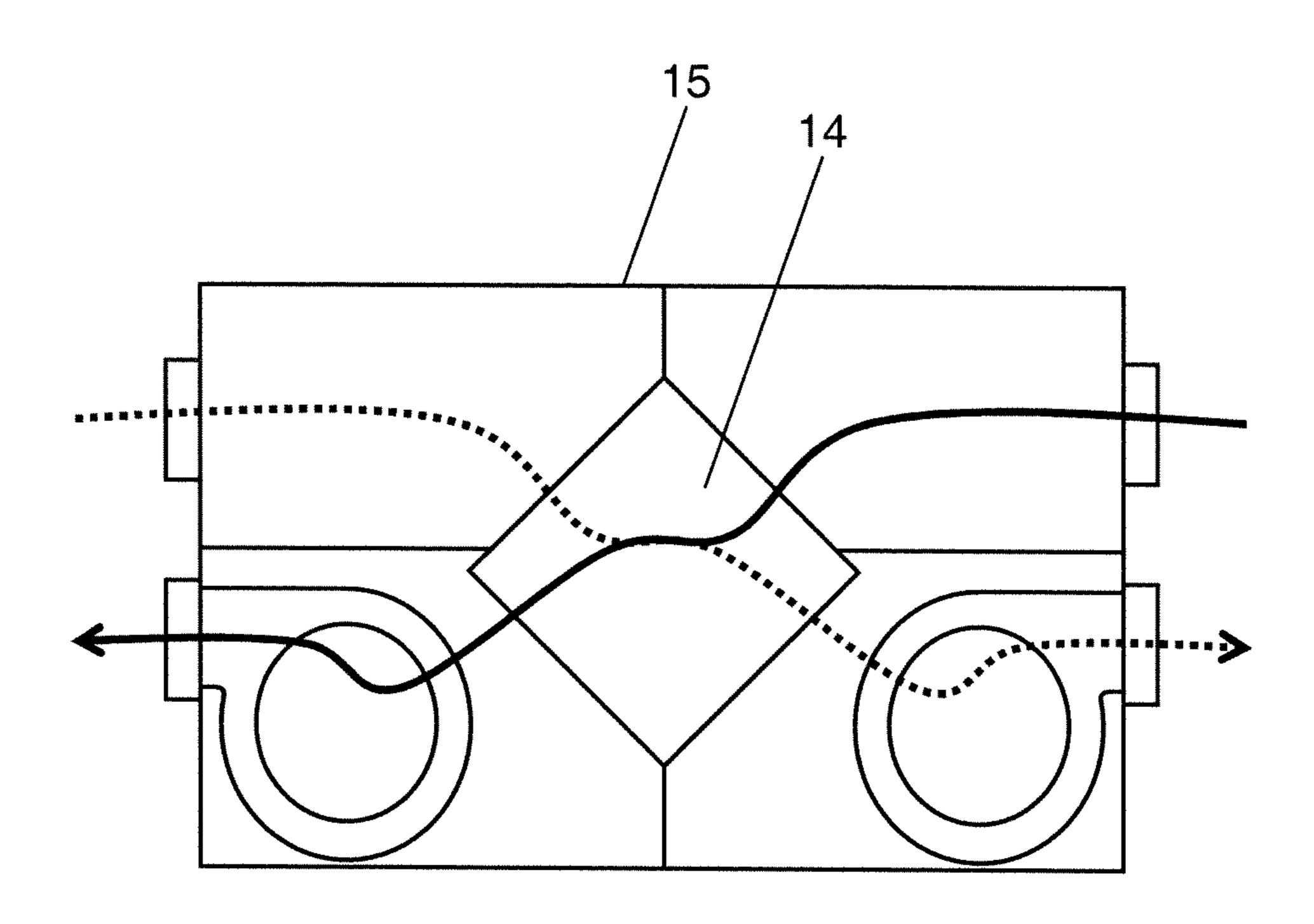
PARTITIONING MEMBER FOR TOTAL HEAT EXCHANGE ELEMENT, TOTAL HEAT EXCHANGE ELEMENT AND TOTAL HEAT **EXCHANGE VENTILATOR USING THE** PARTITIONING MEMBER FOR TOTAL HEAT EXCHANGE ELEMENT
