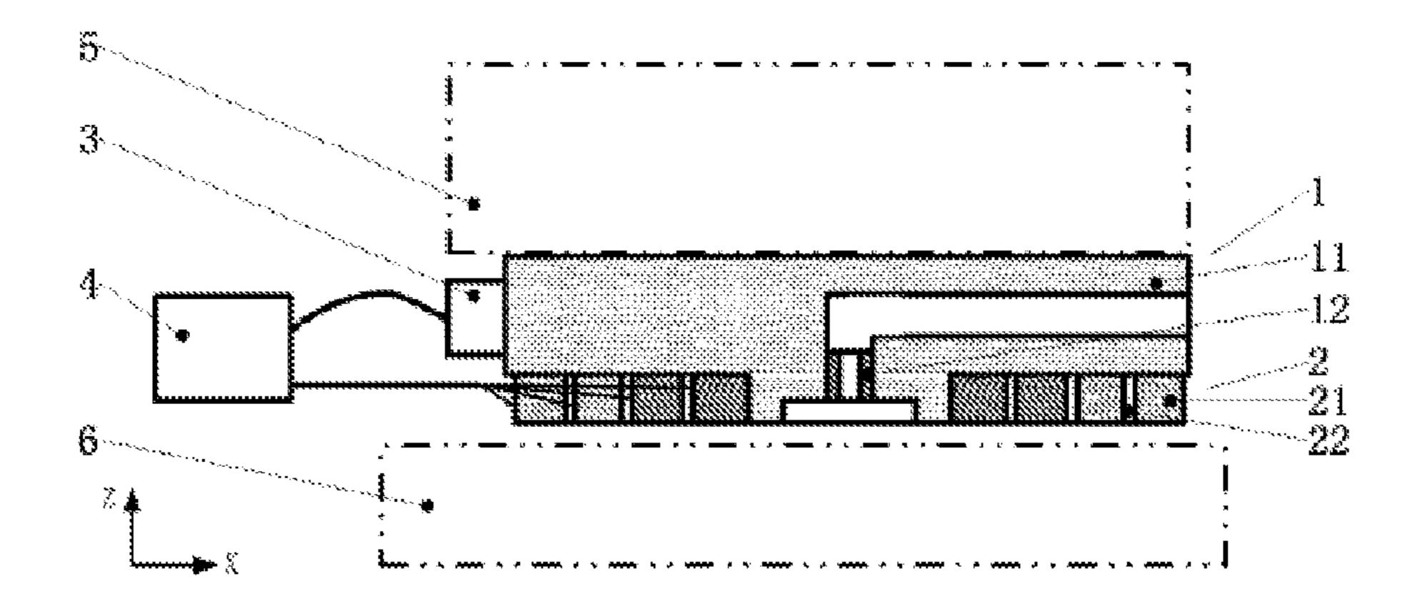
cantly, and the purpose of stabilizing the airbearing is achieved; in addition, the active airbearing device according to the present invention also has the characteristics of a compact structure, convenient operation and control, and high precision, and thus is especially suitable for occasions such as ultra-precision machining or high speed spindle which has high requirements for dynamic stiffness of support.
