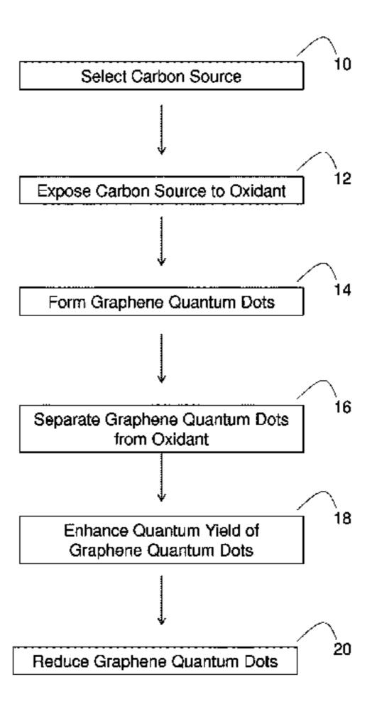
of the present disclosure further comprise a step of enhancing a quantum yield of the graphene quantum dots. In further embodiments, the methods of the present disclosure also include a step of controlling the diameter of the formed graphene quantum dots by selecting the carbon source. In some embodiments, the formed graphene quantum dots comprise oxygen addends or amorphous carbon addends on their edges.
