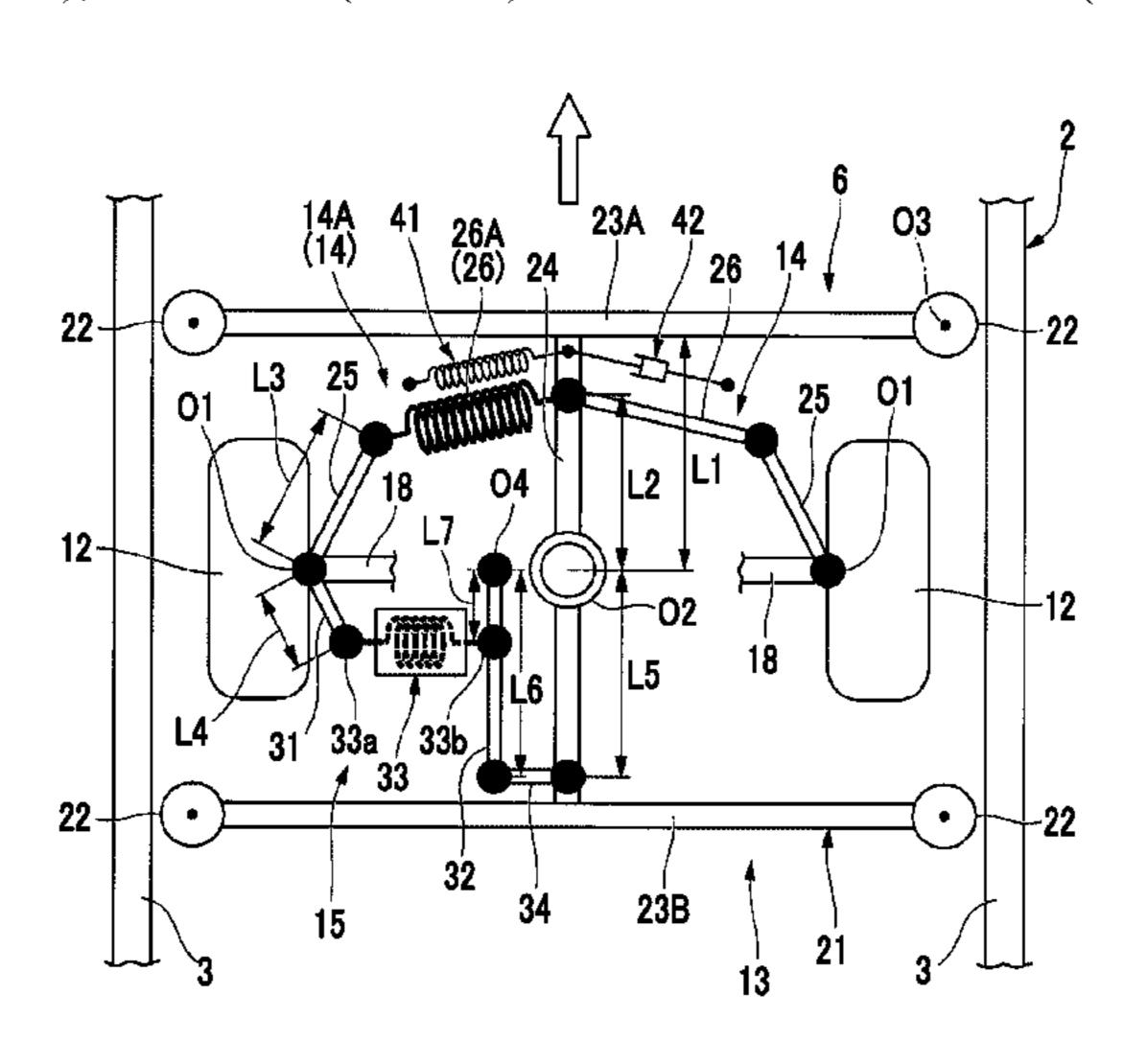
an elastically deformable section connected to the first operation arm and the second operation arm and elastically deformable.
