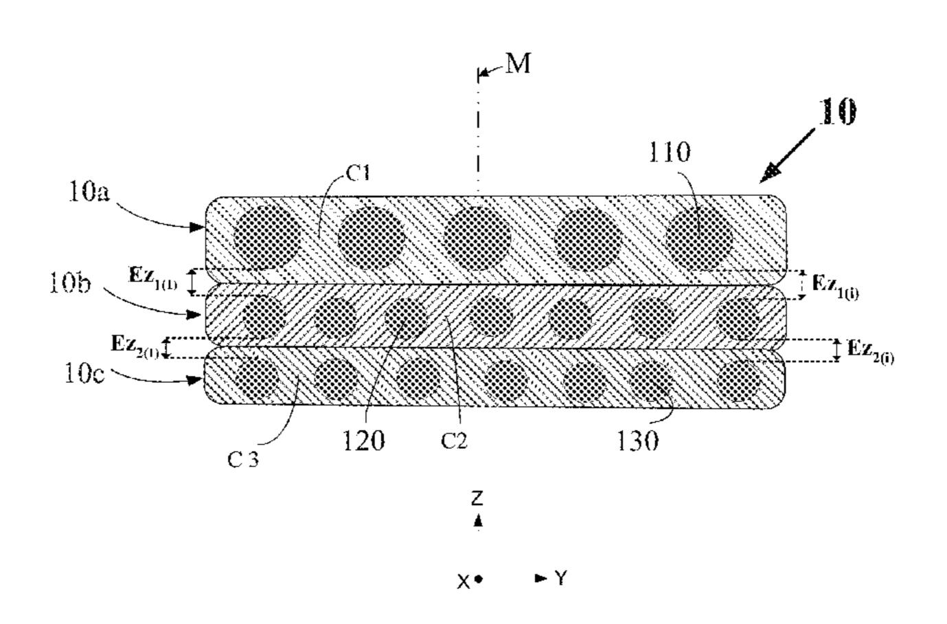
high tensile steel. The first reinforcers have a diameter between 0.40 mm and 0.70 mm and a density between 70 and 130 threads/dm, and the second and third reinforcers have a diameter between 0.20 mm and 0.50 mm and a density between 120 and 180 threads/dm.
