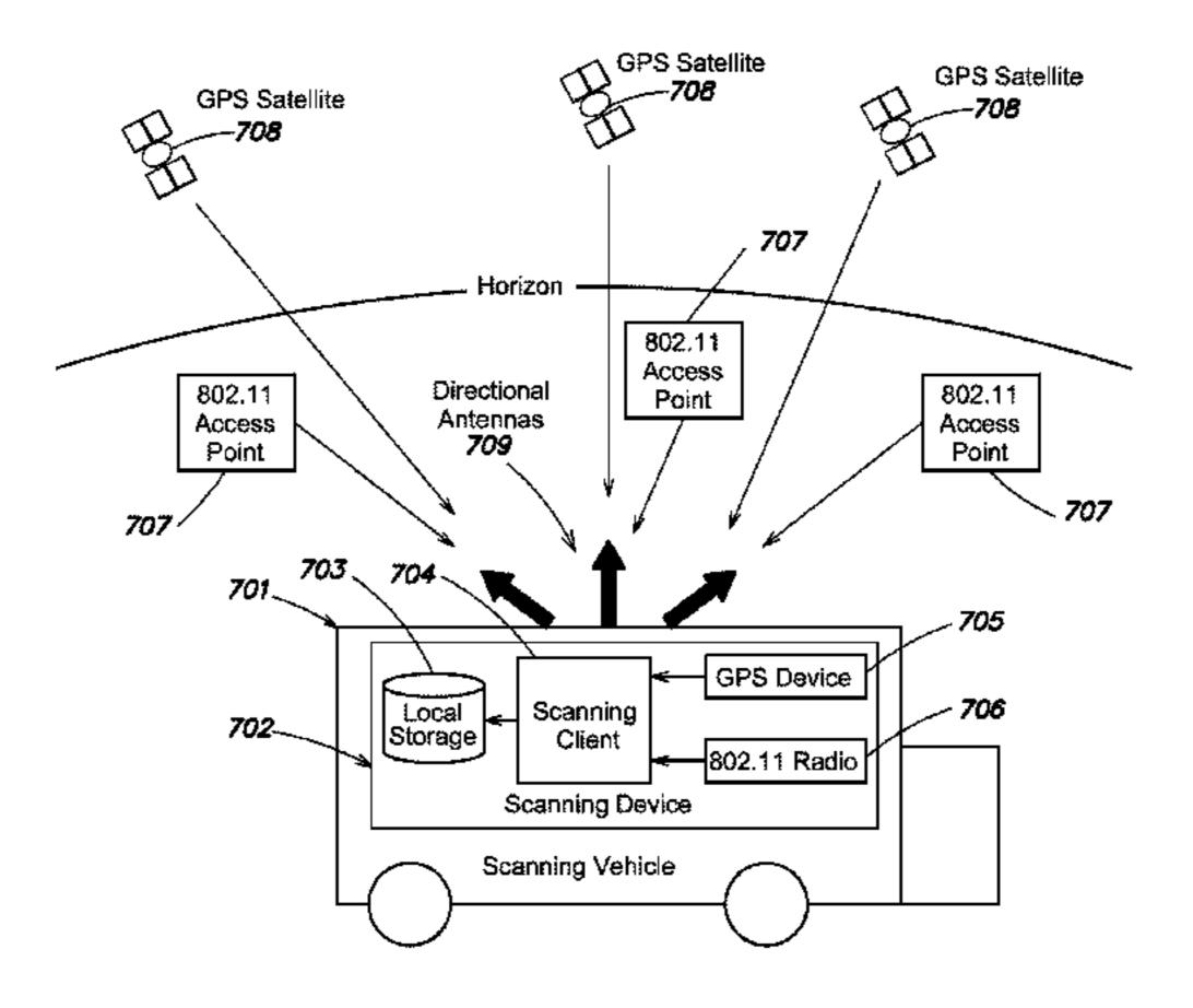
the mobile device using at least the characteristics of signals observed by the mobile device and the location of Wi-Fi access points stored in the reference database, and provides the computed current location to the application or service.
