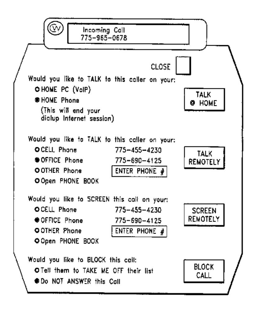
device so that the user can listen to the incoming message and thereby screen the incoming call. Based on the screening, the user can instruct the call management system to connect the caller to the user.
