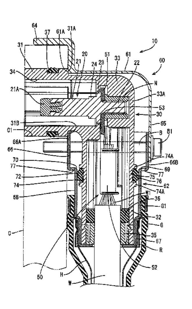
(32) and includes a lower shell (62) for covering the entire outer circumferential surface of the wire introducing portion (32). A seal ring (72) fits on an outer surface of the wire introducing portion (32) and seals between the lower shell (62) and the wire introducing portion (32). Water drainage holes (77) vertically penetrate a stepped portion (69) of the lower shell (62) above the seal ring (72).
