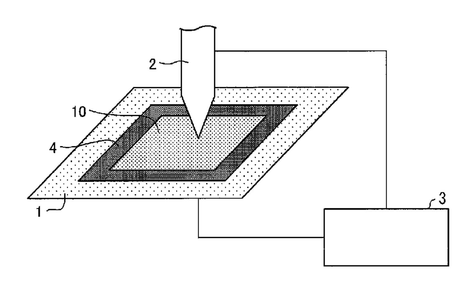
conduction and (b) a test force of the laminate (10) in which a dielectric breakdown occurs, the difference being obtained by subtracting the test force (b) from the test force (a), is measured by use of a nail (2) of N50 specified in JIS A 5508 and under a condition in which the nail (2) descends at a descending speed of 50 µm/min, the difference being not less than 5 N and not more than 50 N.
