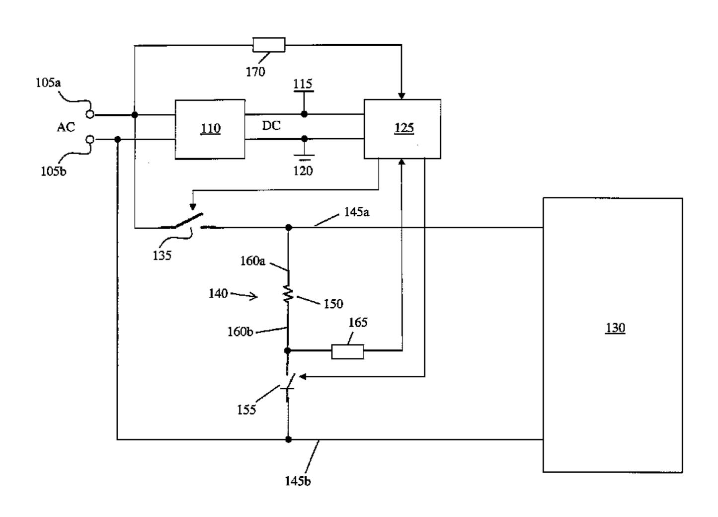
one detected internal electric potential with the first and second reference electric potentials; recognizing a state of good operation or malfunction of the heating circuit (140) in case the at least one detected internal electric potential does not fall within a range of values between the first and second reference electric potentials.
