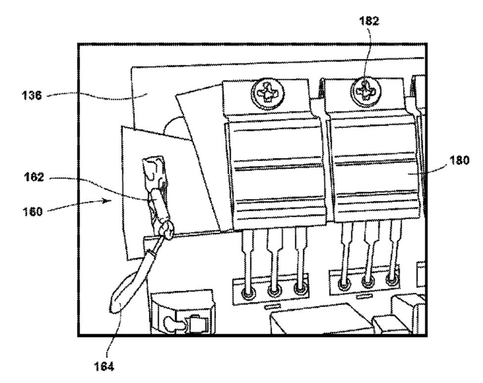
an upper insulating pad is electrically isolated from the heat sink supporting the shield. A damping network electrically connects the capacitive shield to the PCB ground region. Switch-mode power converters are mounted above the upper insulating pad and the shield. The damping network suppresses noise by a parasitic capacitance between the PCB ground region and the heat sink during high frequency power converter operation.
