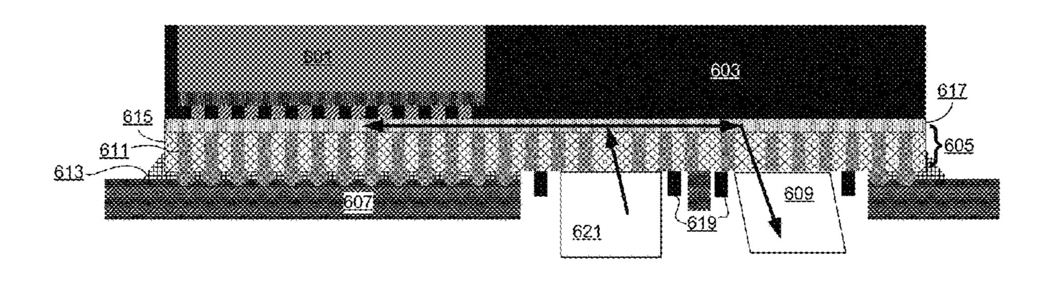
waveguide in the photonic interposer using a grating coupler.
