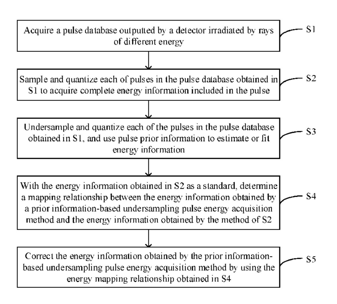
determining a mapping relationship between 10 the energy information obtained by a prior information-based undersampling pulse energy acquisition method and the energy information obtained by the method of S2; and S5 correcting the energy information obtained by the prior information-based undersampling pulse energy acquisition method by using the energy mapping relationship obtained in S4.
