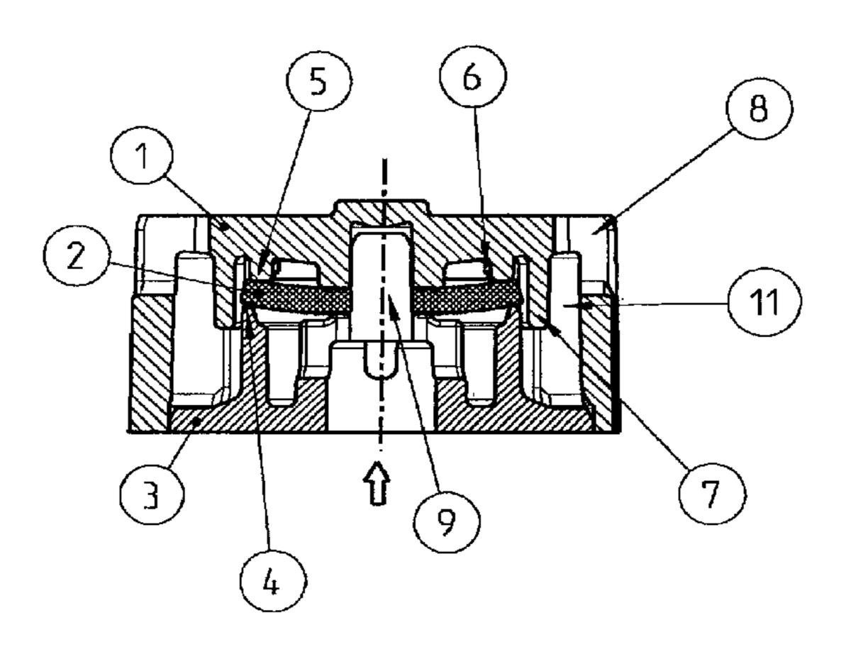
pressure gradient between an inlet space and an outlet space or atmosphere and to open a flow cross section between the inlet space and the outlet space or atmosphere, in which, as viewed in the circumferential direction of the diaphragm disk, a plurality of hold-downs which are arranged at a circumferential spacing from one another and hold down the radially outer region of the diaphragm disk locally against the valve seat are provided on the valve housing.
