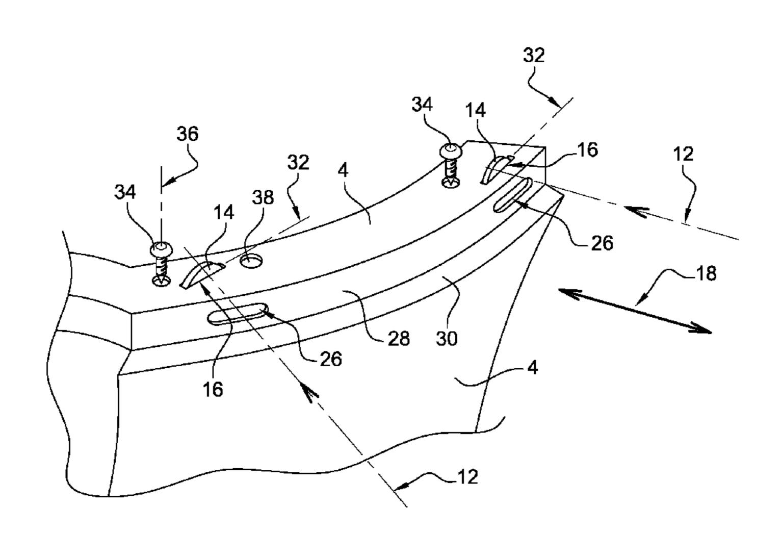
a translation coupling element for the translation member and the fixed bodywork panel engaging the through hole, so that moving the translation member along the member translation axis causes a translation of the fixed bodywork panel relative to the support part in a translation direction allowing the fixed bodywork panel to be in a desired position, e.g. flush with a mobile bodywork panel.
