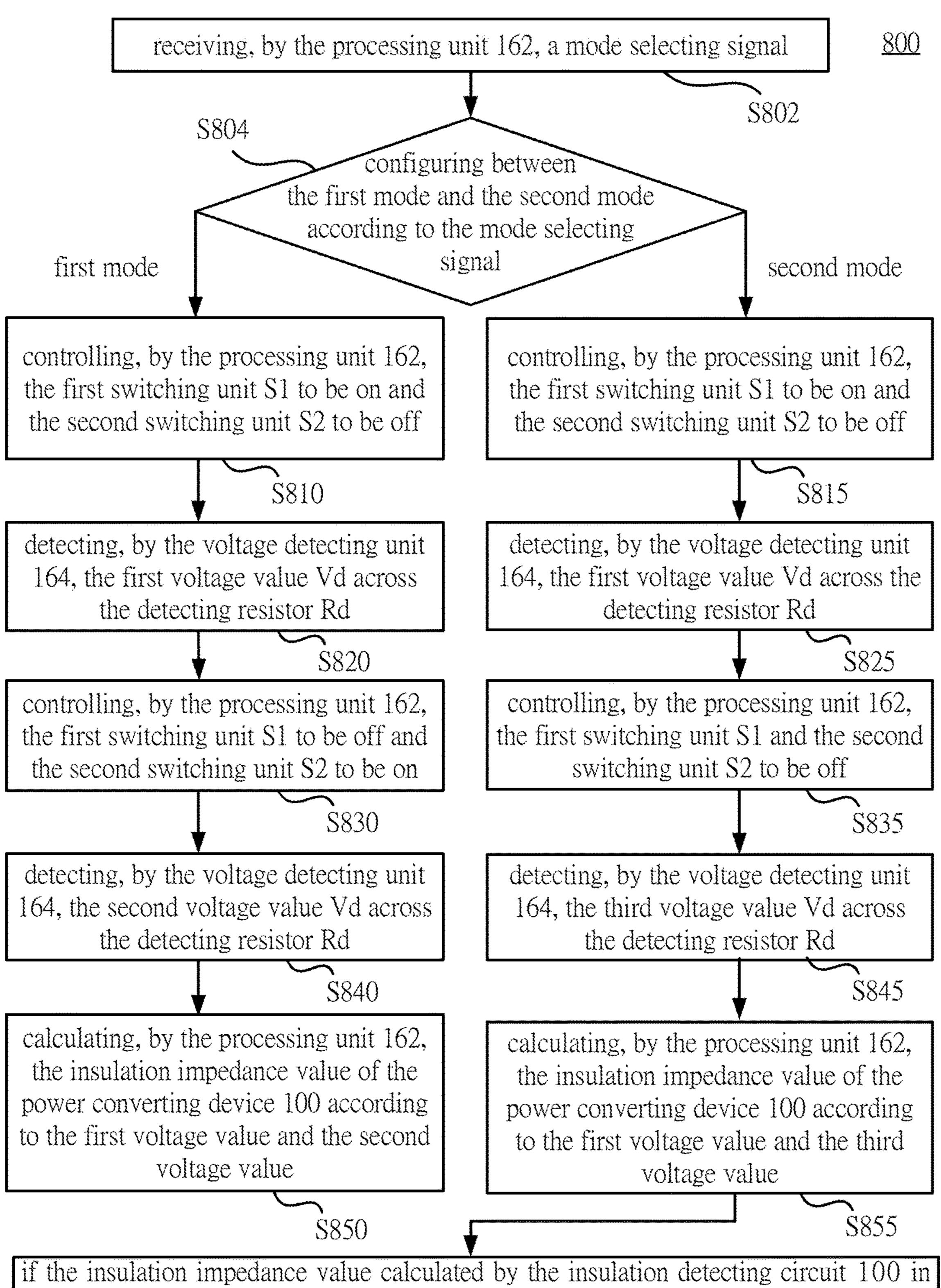
if the insulation impedance value calculated by the insulation detecting circuit 100 in the second mode is smaller than a predetermined value or if the difference between the first voltage value and the third voltage value is smaller than a predetermined voltage value, switching to the first mode and calculating the insulation impedance value
