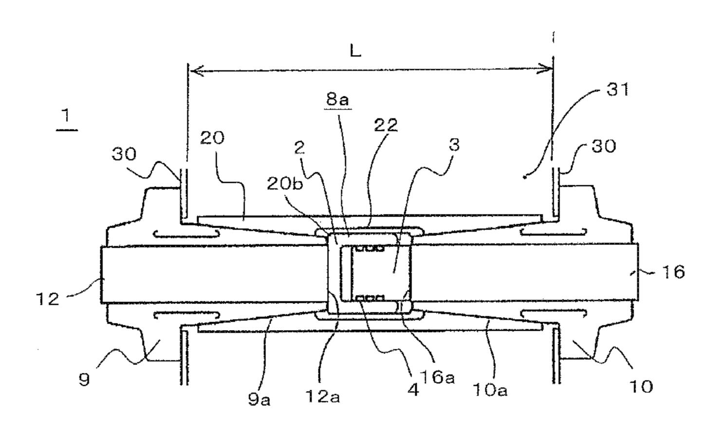
adapter surrounds the nose of the first bushing, the nose of the second bushing, and the connection element as one.
