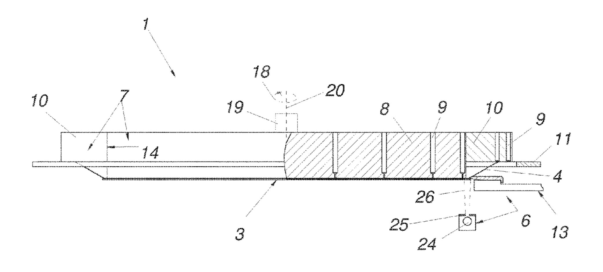
detach the reinforcement edge in one piece from the carrier film stretched by interaction of clamping device and support.
