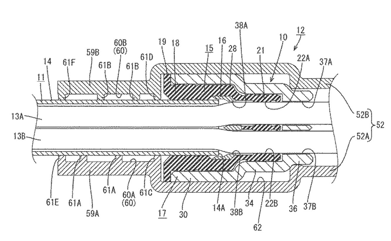
sheath and first to fourth through holes through which the first to the fourth electric wires are passed, respectively. The cap is fitted on the rubber stopper and presses the rubber stopper inward. The holder includes a sheath holding portion for holding the sheath and a cap holding portion for holding the cap.
