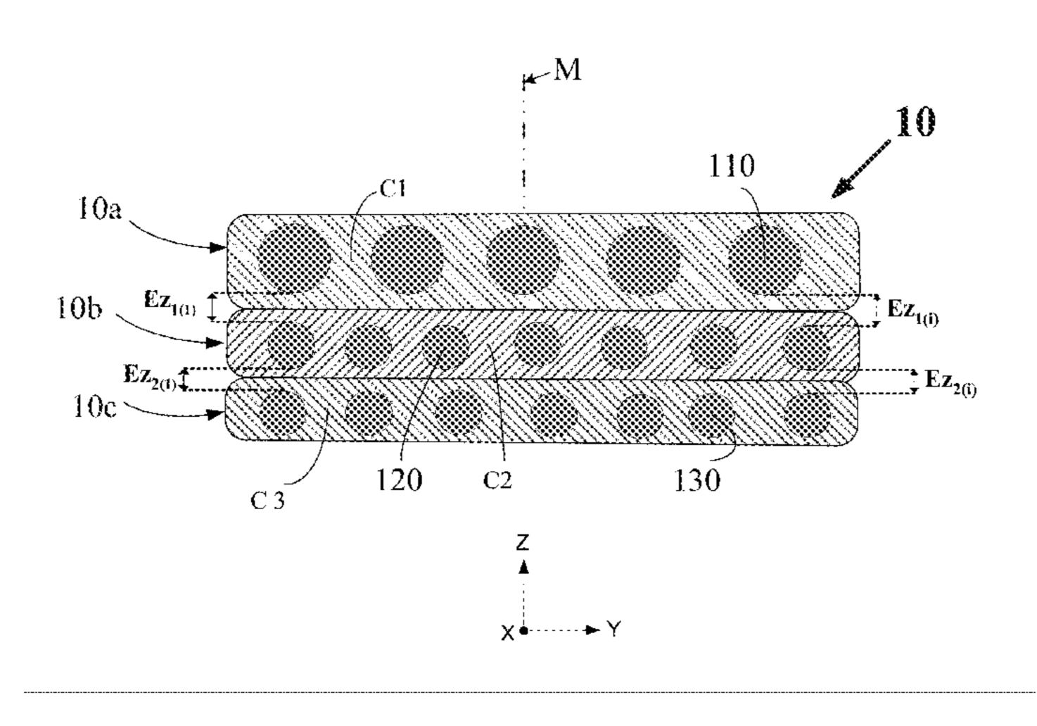
forcers, which are monofilaments of high tensile steel. The first reinforcers have a diameter between 0.40 mm and 0.70 mm and a density between 70 and 130 threads/dm, and the second and third reinforcers have a diameter between 0.20 mm and 0.50 mm and a density between 120 and 180 threads/dm.
