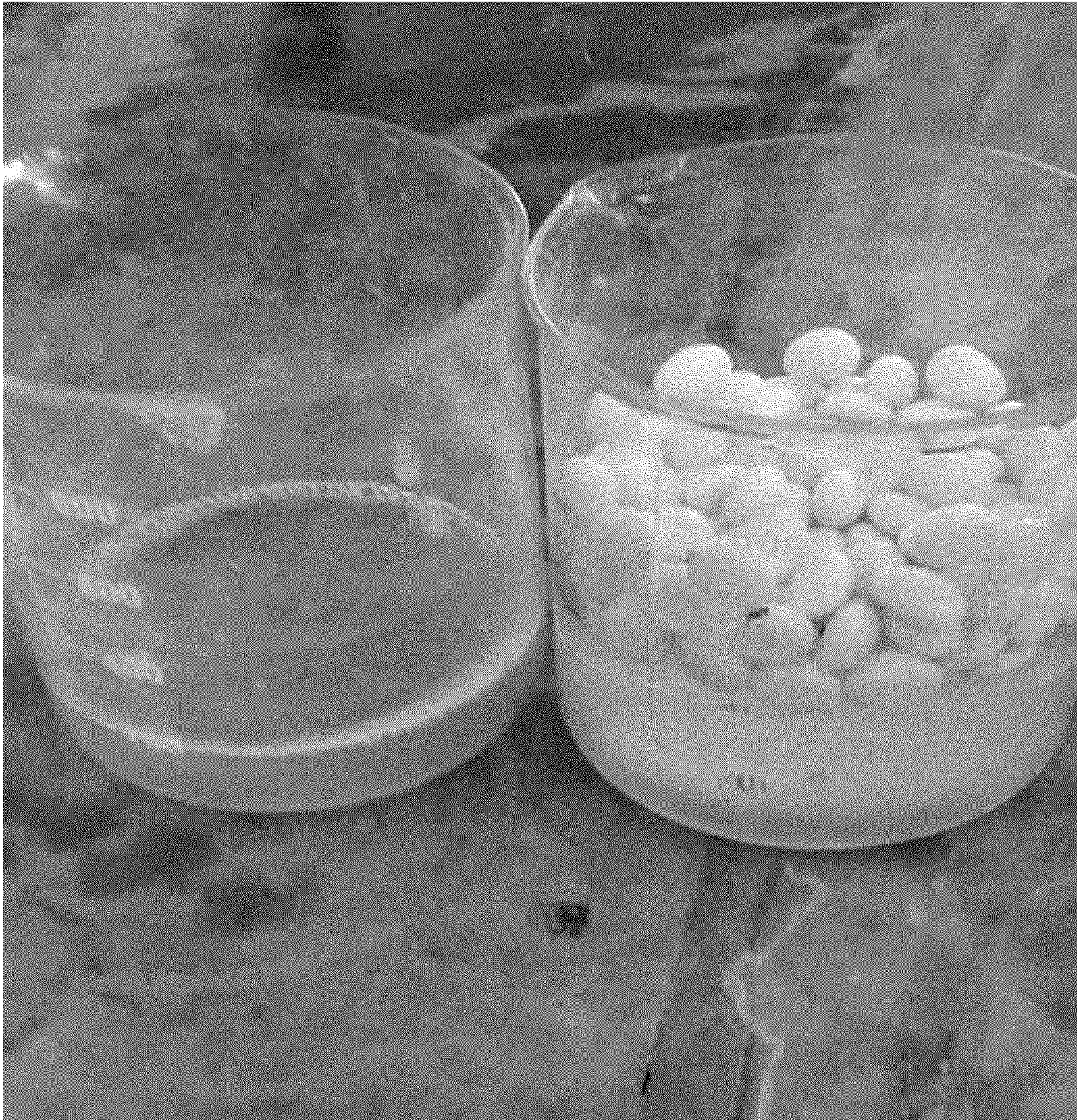
Figure 12: Effect of beads on water evaporation
