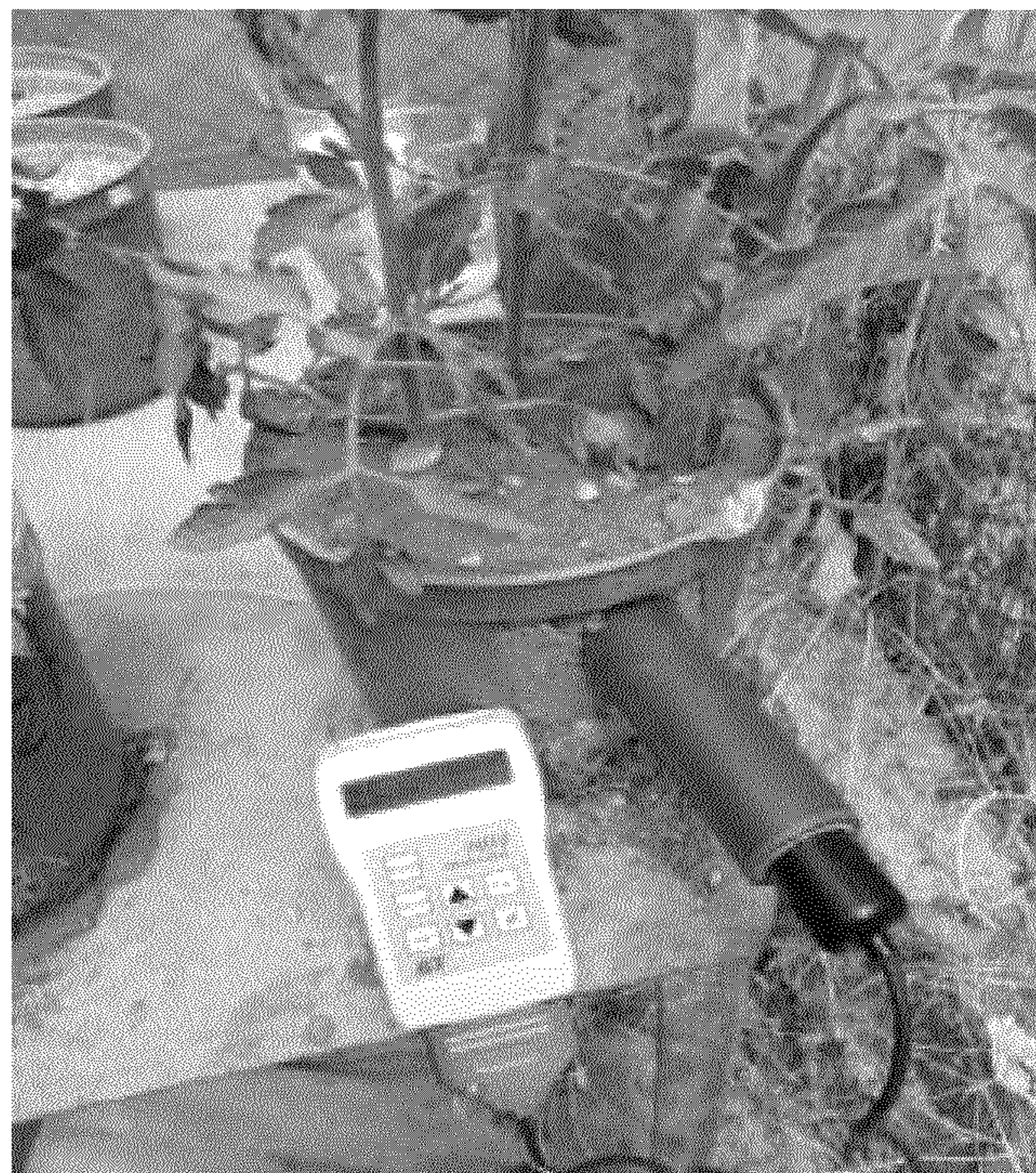
Figure 5 : Soil moisture measurement above beads layer.
