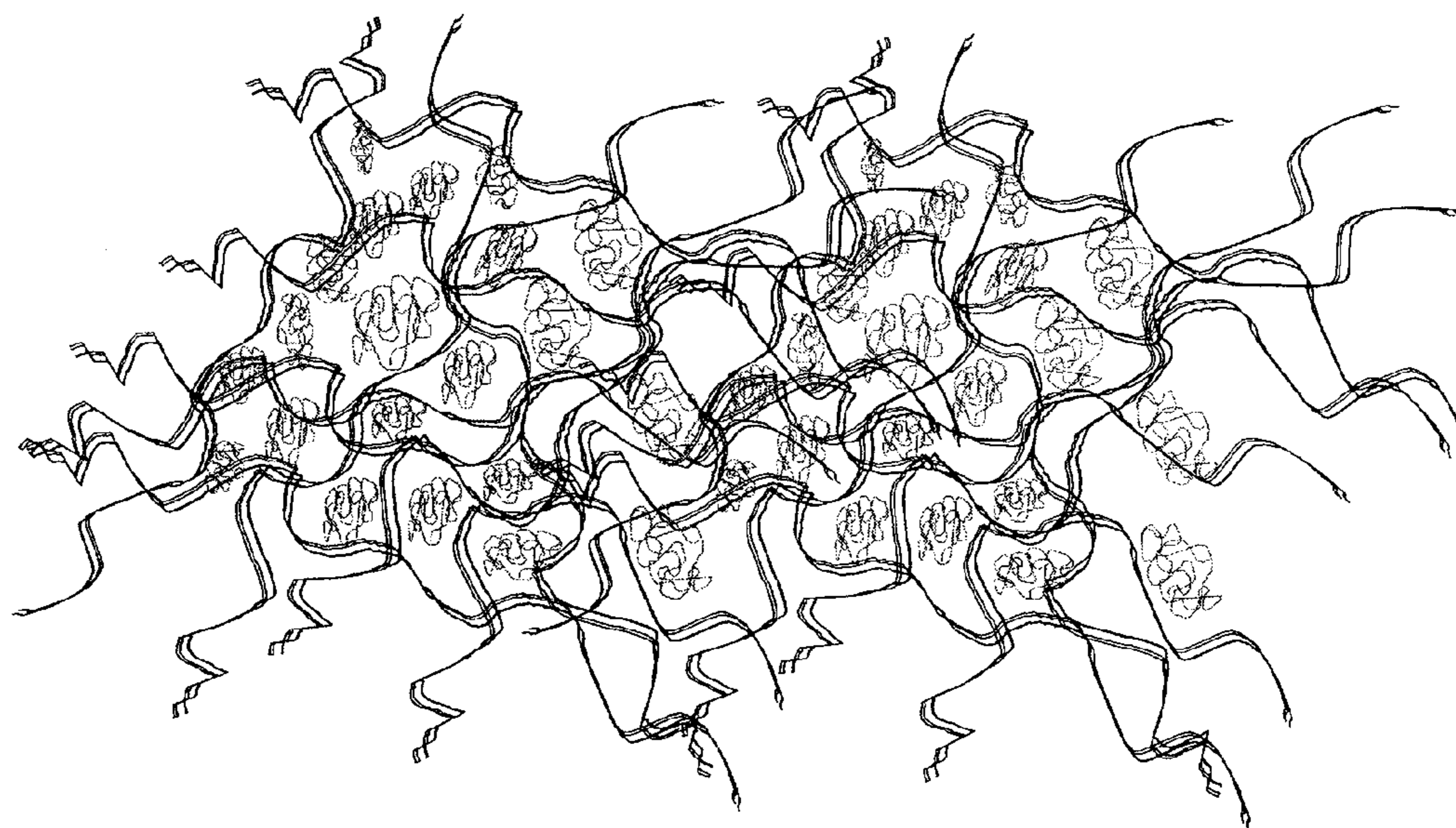
Figure 3: Schematic of GELPEO formed through aqueous PEO assisted regeneration of cellulose.
