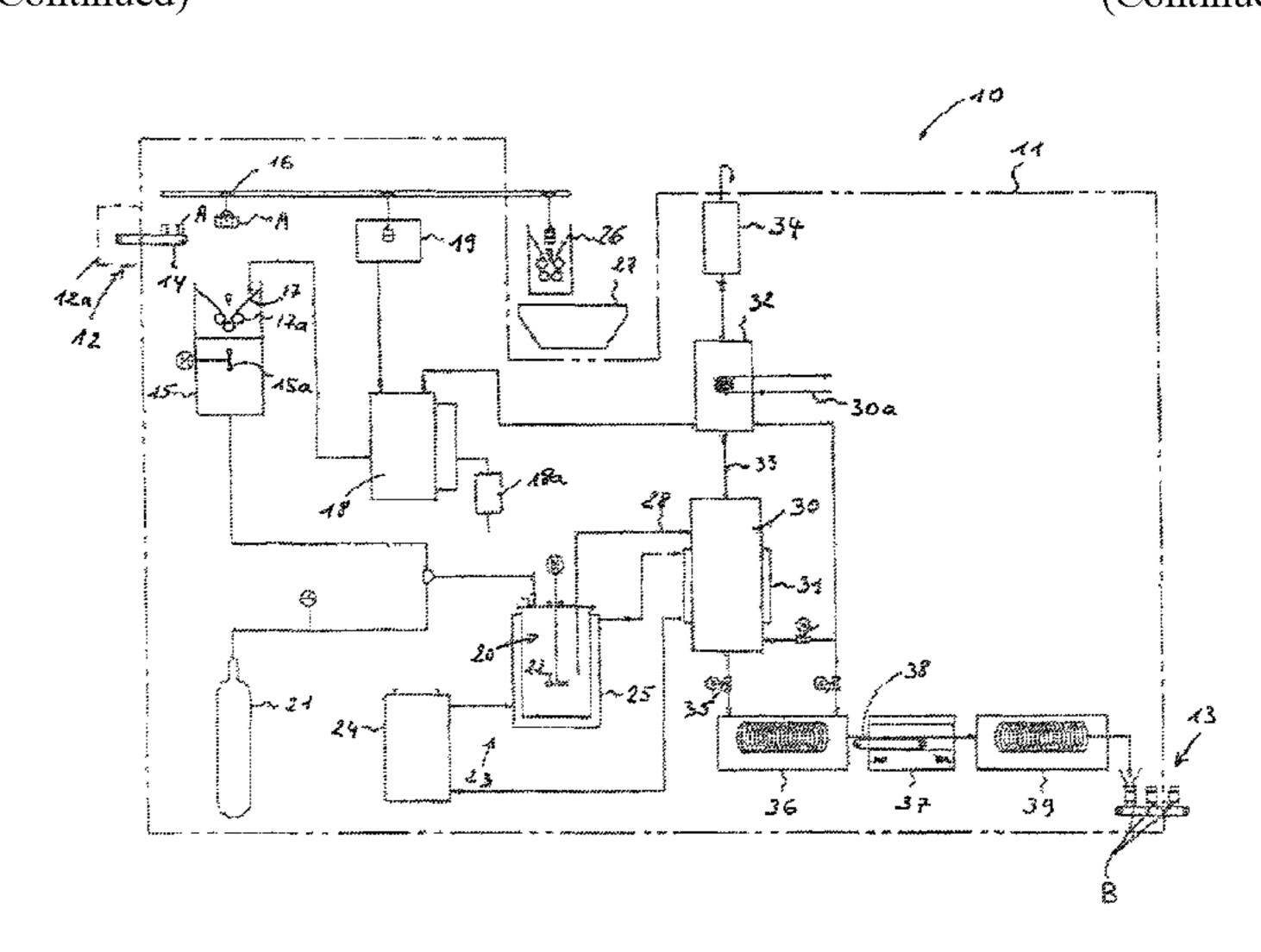
transferring the solution and/or liquid suspension into the pressure reactor, and a device for introducing an oxygen atmosphere into the pressure reactor and for pressurizing the atmosphere. A heating mechanism is provided for subjecting the contents of the pressure reactor to heat treatment at a temperature between 150° and 350° C. to complete the wet-route oxidation.
