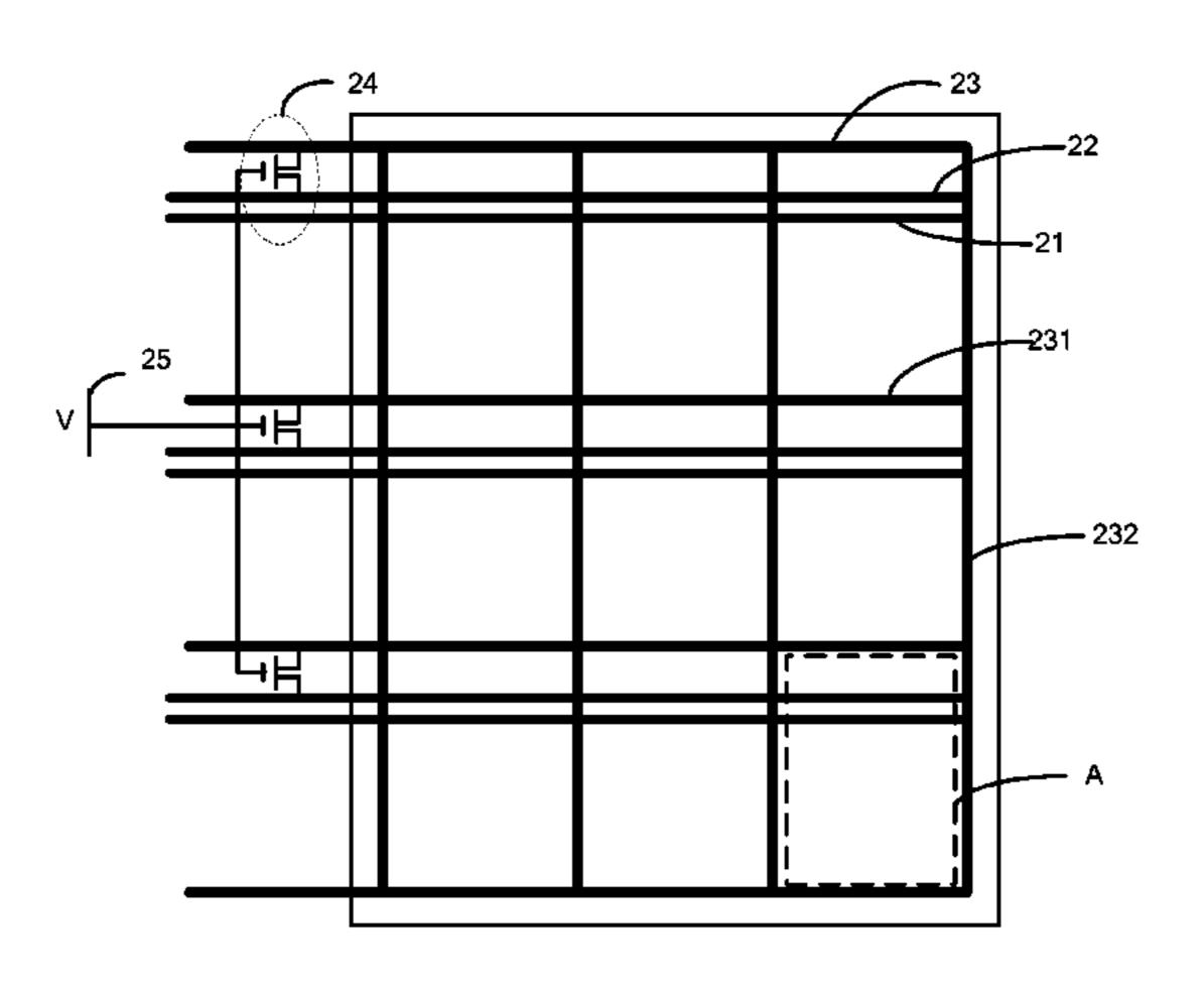
thus a total resistance of the VDD lines and the VDD grid connected in parallel is decreased relative to the own resistance of the VDD line, so as to reduce the voltage drop on the VDD line in a direction in which the scanning control lines extend, and in turn to decrease a variation in a OLED driving voltage signal effectively, ensuring uniformity of luminance across the display area.
