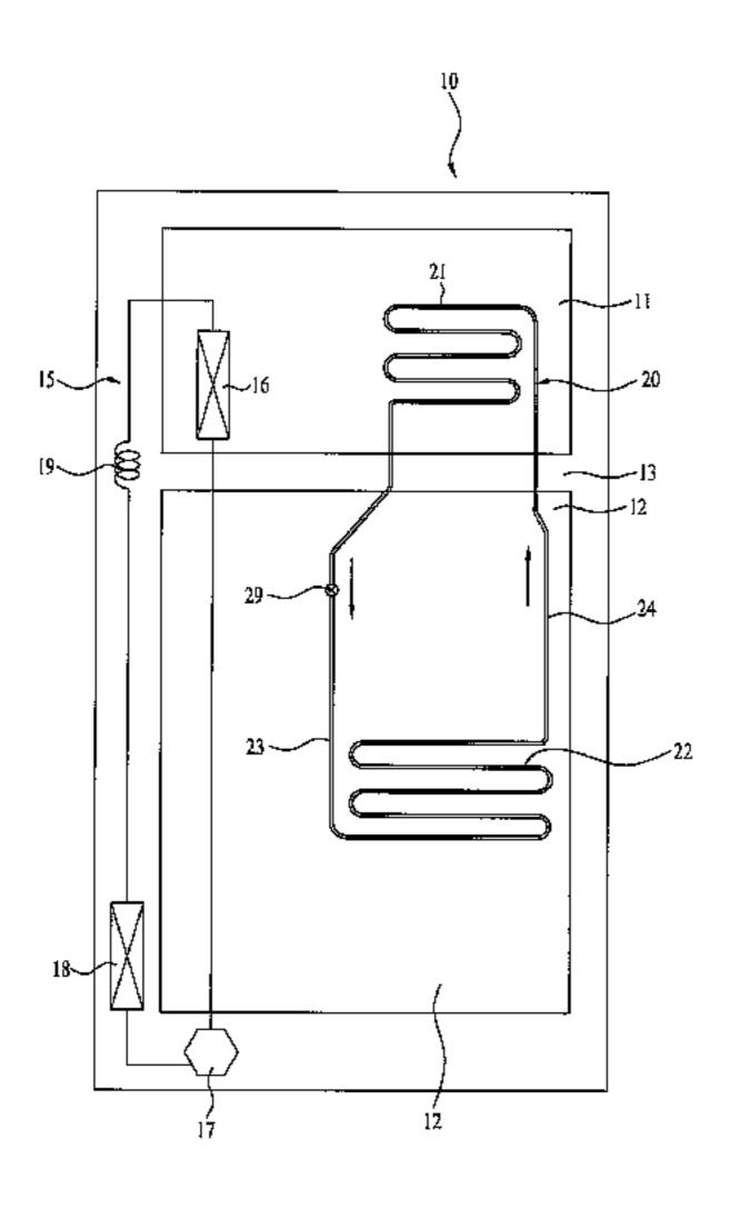
switching circuit provided between the valve and the electrical power storage device. When the power source does not supply power to the cooling circuit, the control circuit may operate the thermosyphon using power stored in the electrical power storage device.
