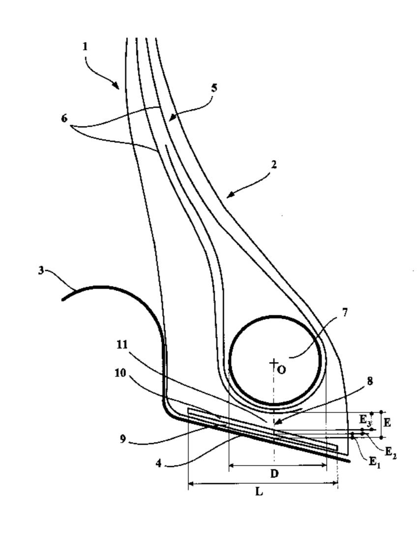
wire (7), having a shear stiffness  $K_3$  at most equal to 0.3 times the shear stiffness  $K_1$  of the surface layer (9).
