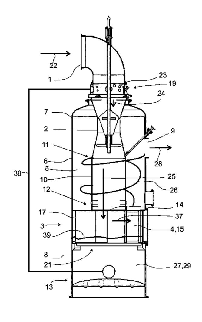
second vertical cylindrical vessel and the swirl generator are arranged in a vertical cylindrical separation space of a first vertical cylindrical vessel. The swirl generator is arranged above the liquid tank.
