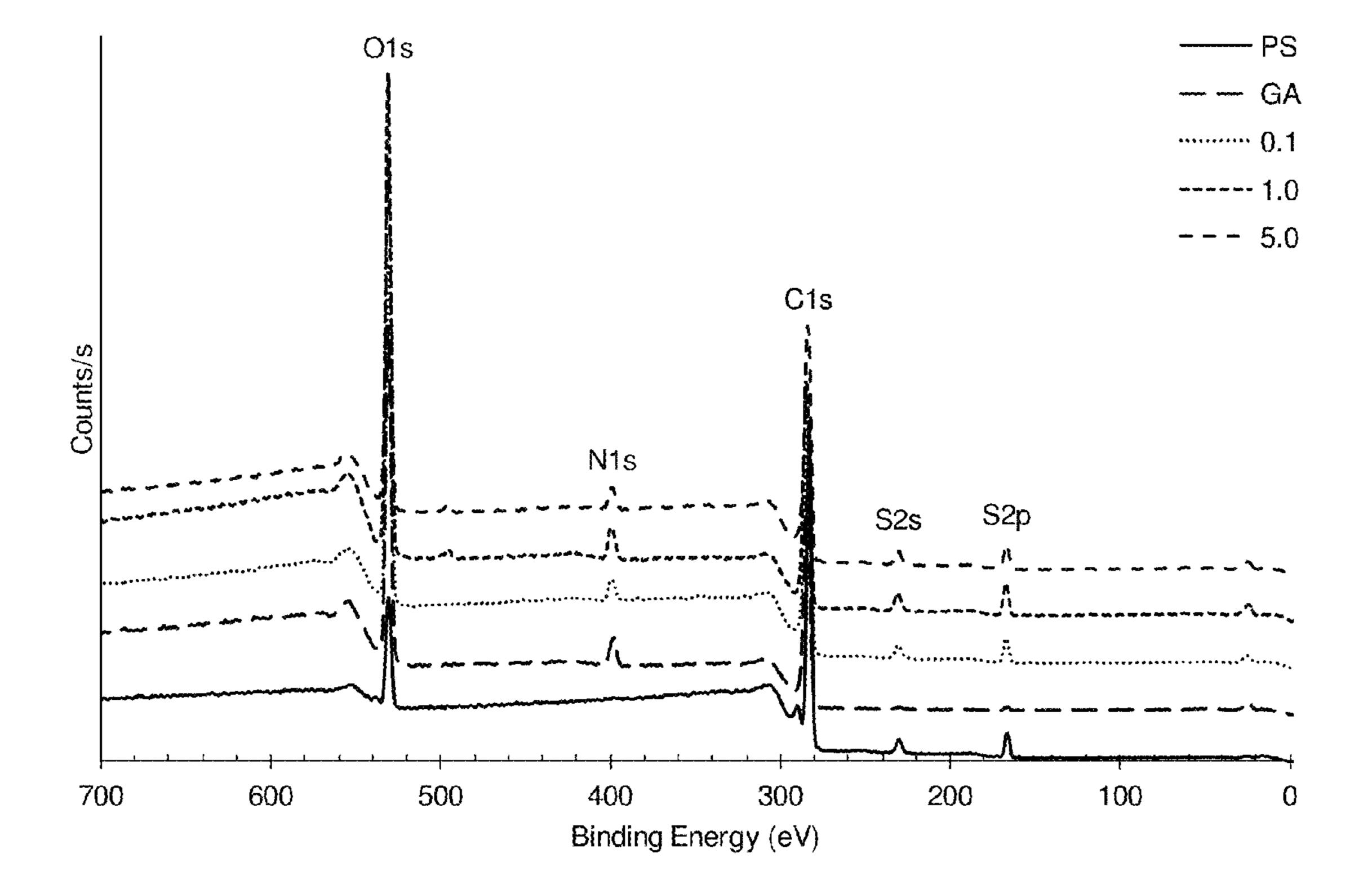
XPS survey spectra of polysulfone surfaces modified with chitooligosaccharide, gallic acid, and different levels of heparin.
