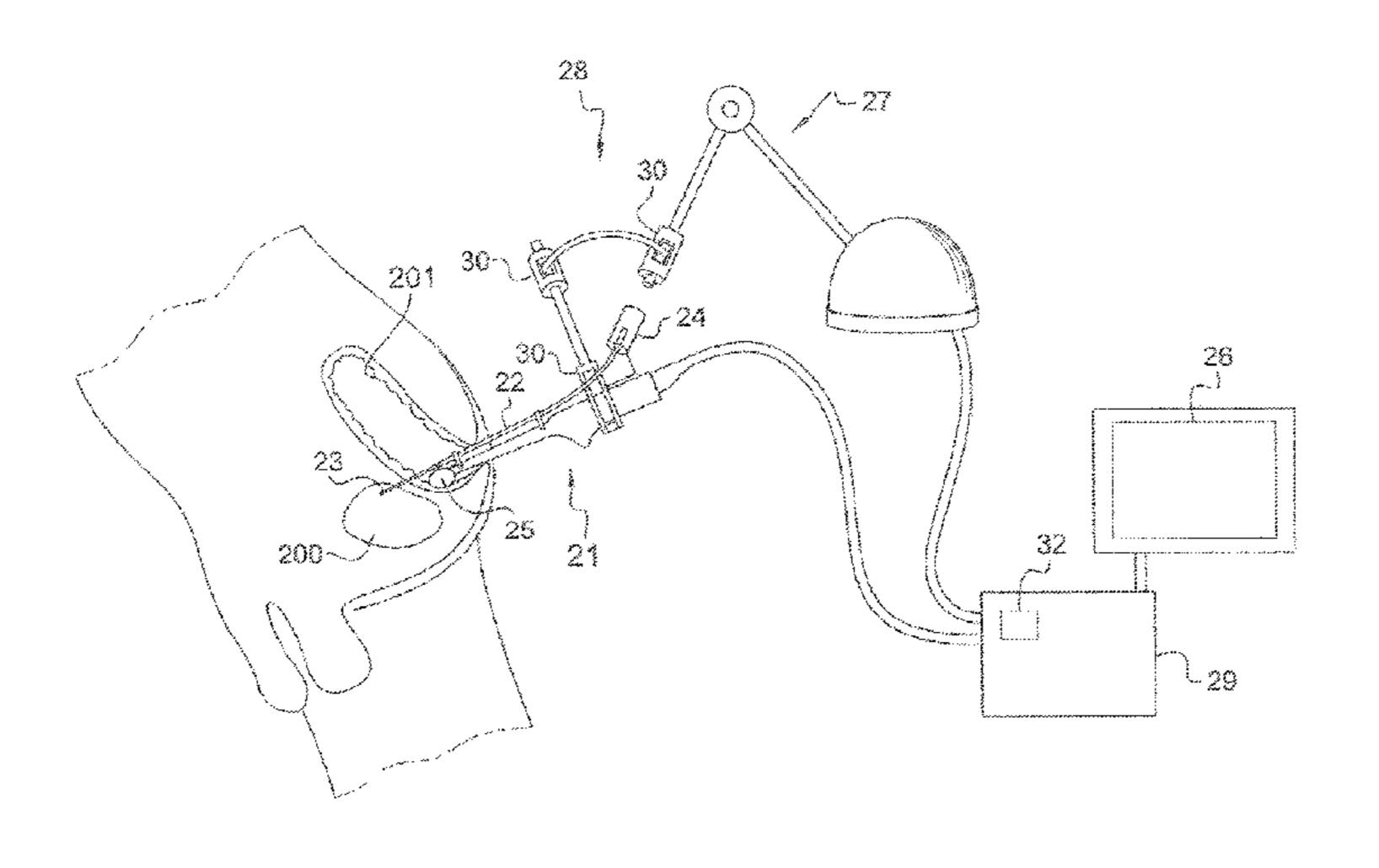
of freedom, a blockage imposed on the degree of freedom can be released when an outer stress exerted on the instrument (2) exceeds a predetermined threshold.
