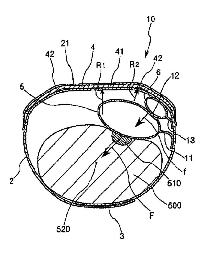
at least a portion thereof overlaps with the balloon and which is adapted for pressing against the balloon. The device provides an excellent hemostatic effect and prevents numbness and poor circulation in areas peripheral to the site of attachment.
