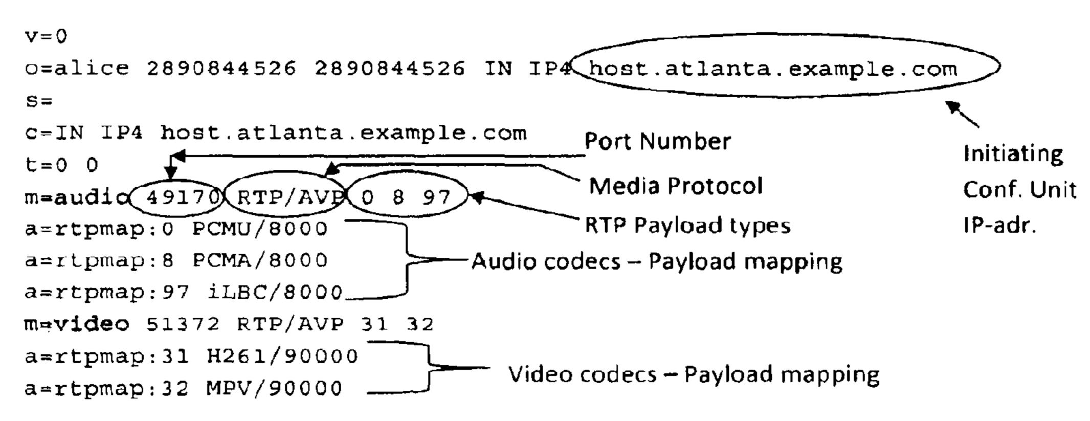
Figure 3 illustrates an example of data information exchanged between two conference units when setting up an Audio media line and a Video Media Line.
