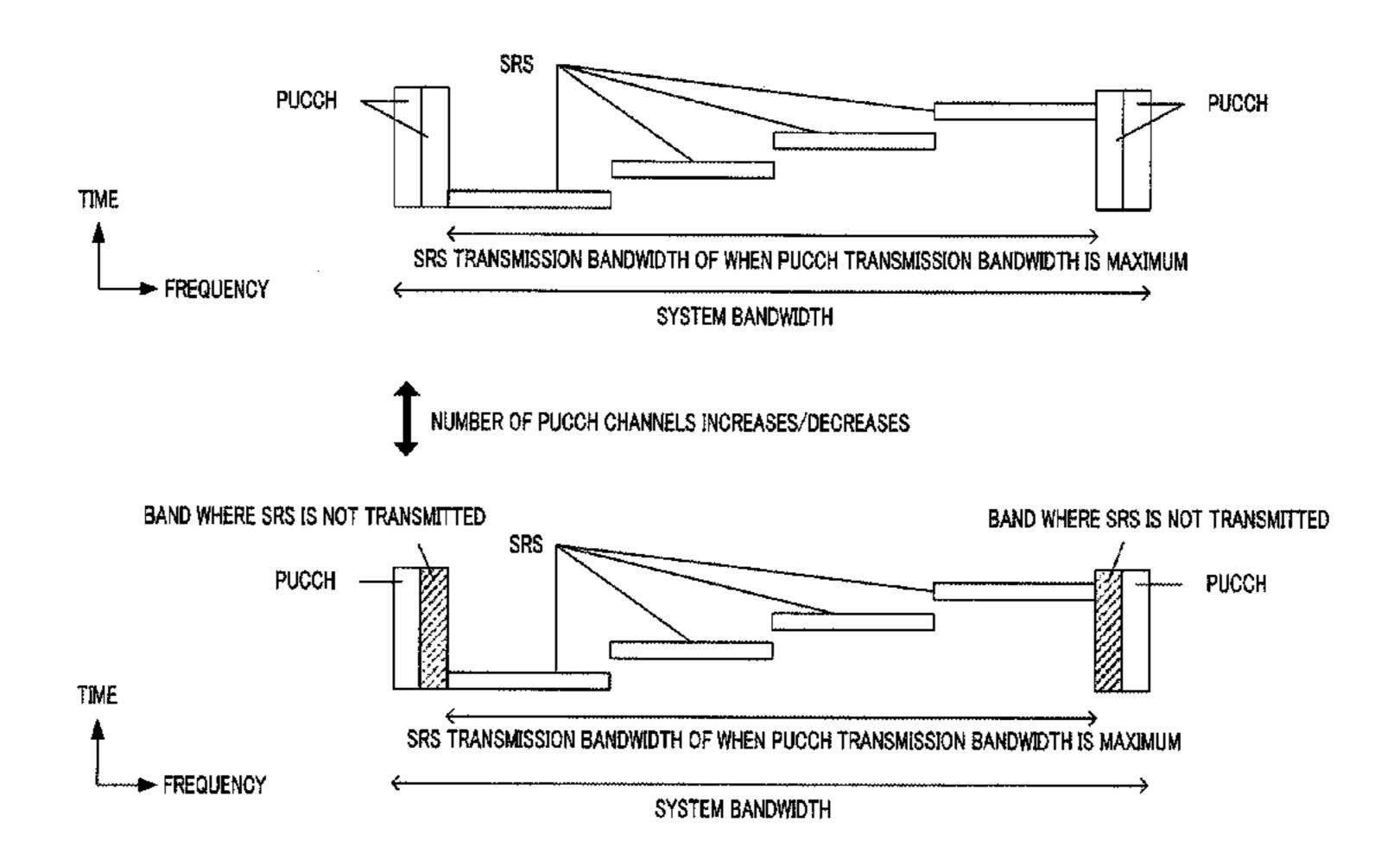
reference signal transmission bandwidth according to the SRS arrangement information transmitted from the base station and furthermore controls the transmission interval of the frequency-multiplexed SRS.
