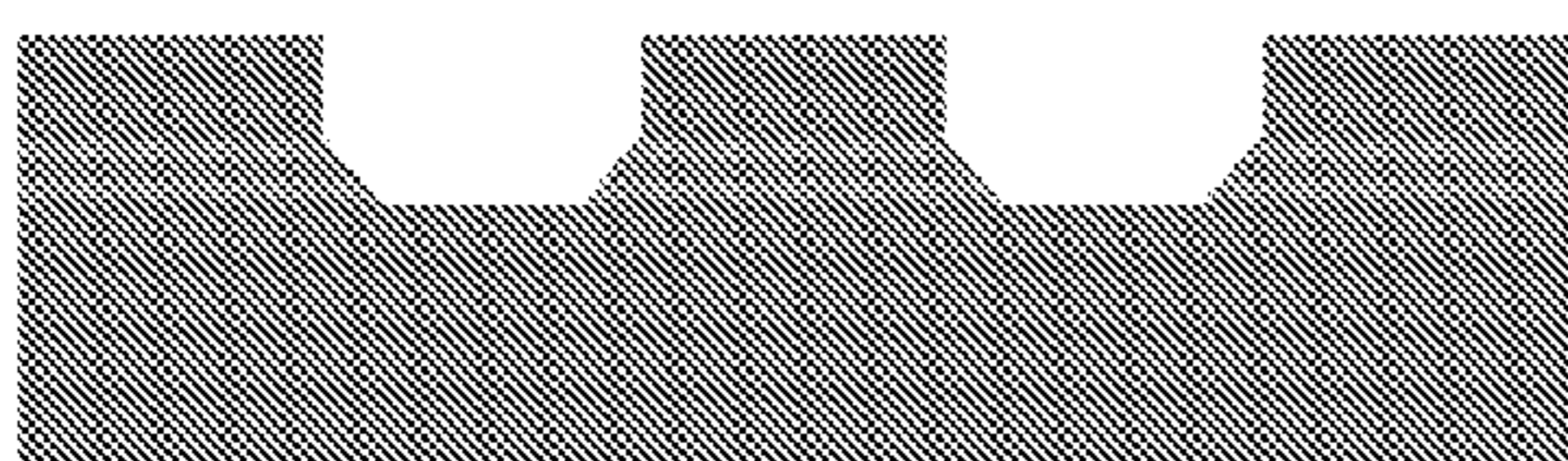
SiO 2 etch in BOE solution
