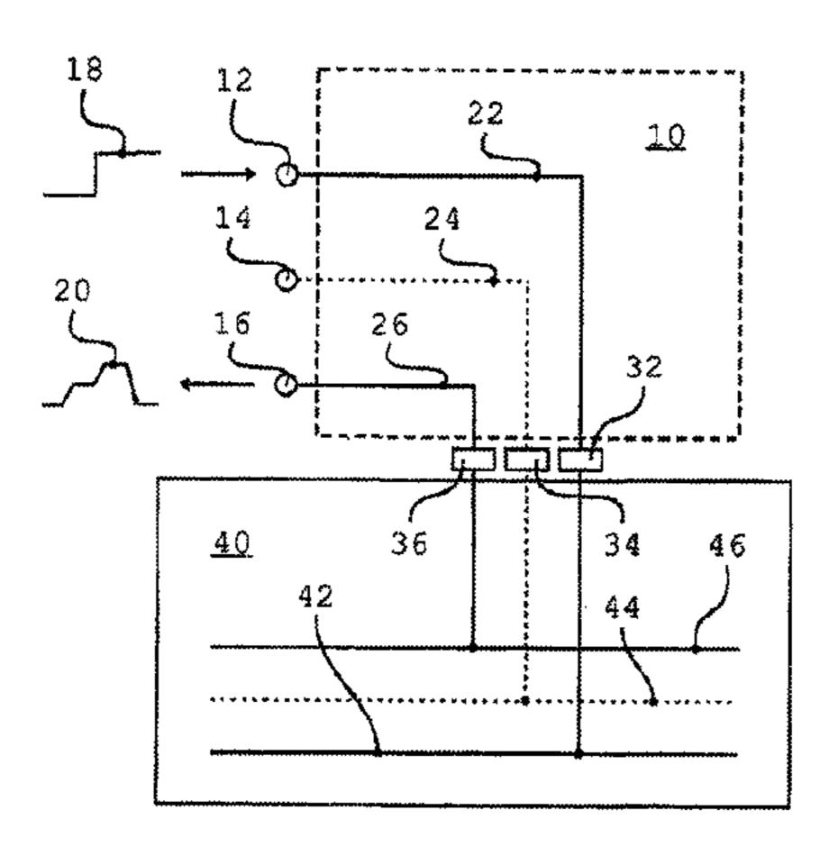
if there is a deviation between the near end crosstalk signal and the corresponding reference signal pattern, an information that there is any defect in the electric device is displayed.
